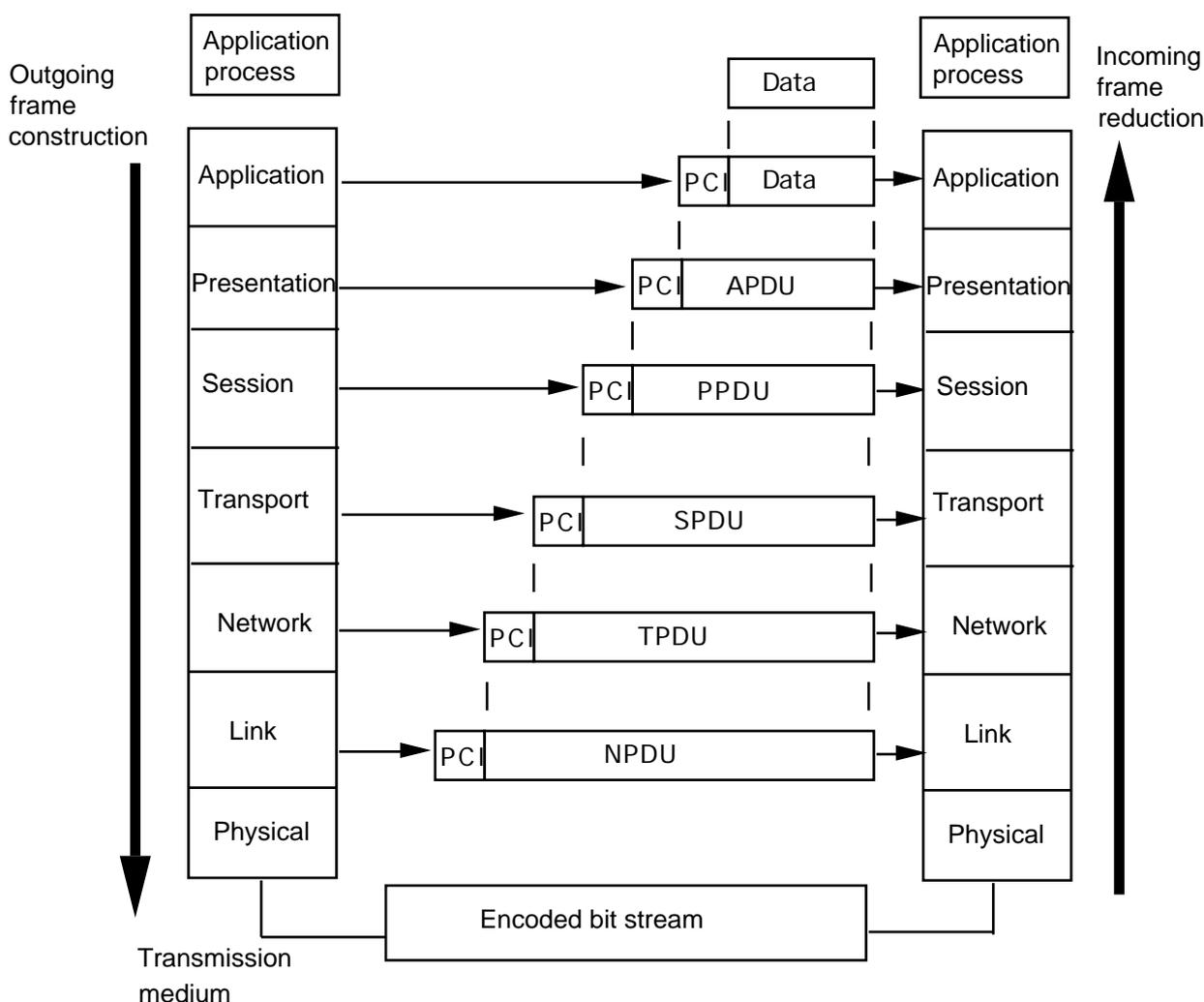
Figure 2. An excerpt of the existing lecture notes to illustrate the ISO Reference Model for Open Systems Interconnection.
