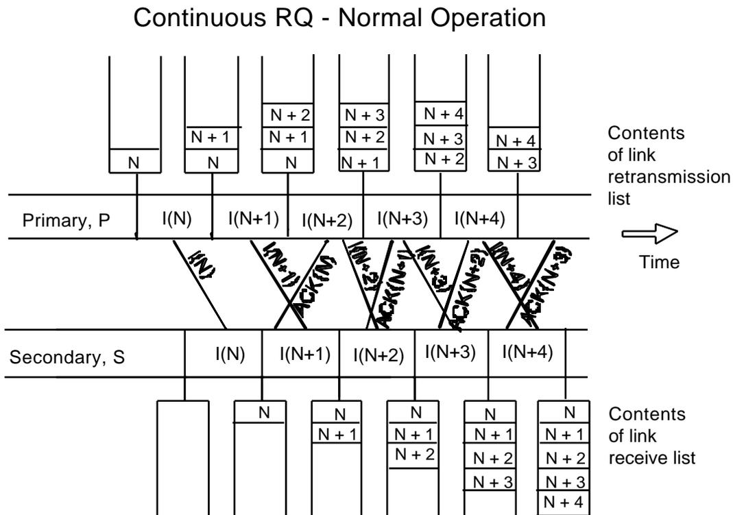
Figure 1. Continuous RQ Error Control Scheme.
