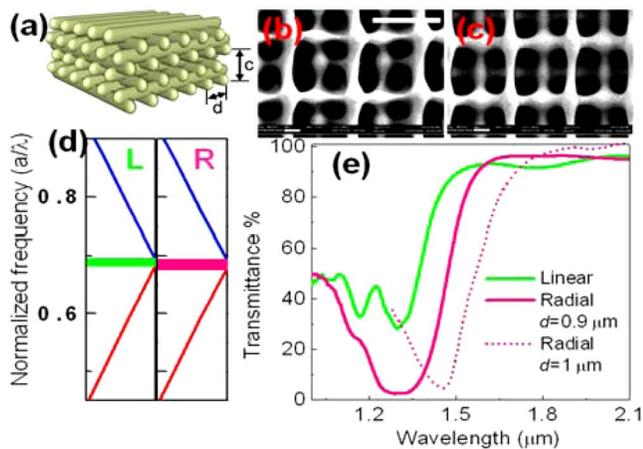
Fig. 4. (Color online) (a) Schematic of the woodpile PC. (b), (c) SEM images of PCs fabricated with (b) the linearly and (c) radially polarized beam illumination. Scale bar: 900 nm. (d) Calculated band diagrams in the  $\Gamma$ -X direction of structures in (b) and (c). (e) FTIR measured transmission spectra (solid curves) of PCs in (b) and (c) and another PC with different lattice constant ( $d=0.95 \mu\text{m}$ ) fabricated with a radially polarized beam.
