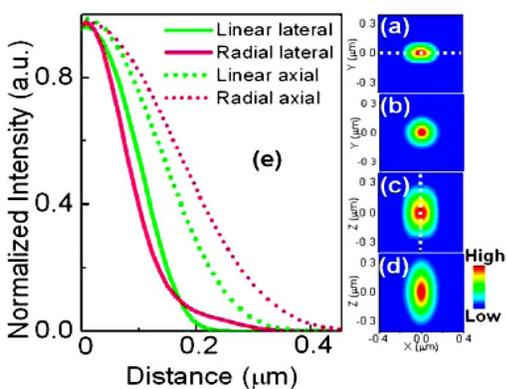
Fig. 2. (Color online) Calculated two-photon intensity distributions along (a),(b) the transverse and (c),(d) the axial directions in the focal region of an objective with NA=1.4 through the coverglass ( $n_1=1.515$ ) and Ormocer ( $n=1.47$ ) interface under (a),(c) linearly polarized beam illumination and (b),(d) radially polarized beam illumination. (e) The cross section comparison of the focal spots along the  $X$  and the  $Z$  directions.
