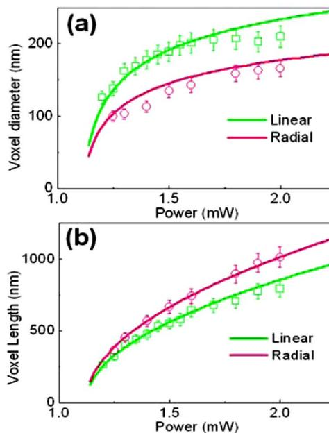
Fig. 3. (Color online) Predicted (solid curve) and measured (dots and squares) (a) voxel diameter and (b) voxel length as functions of the laser power for a constant exposure time of  $t=5$  ms.
