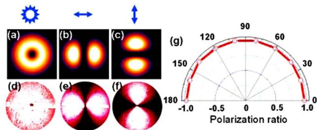
Fig. 1. (Color online) Simulated profiles of (a) a radially polarized beam and its (b) horizontal and (c) vertical polarization components before being focused by the fabrication objective. (d)–(f) Experimentally obtained profiles corresponding to (a)–(c), respectively. (d) The polarization ratio of the radially polarized beam in different polarization directions.
