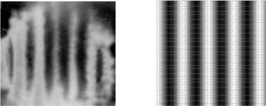
Figure 2. Magneto-convective instability: liquid crystal visualization (left) and the computed three-dimensional temperature field near the cold wall (right) for  $(Gr_m, Gr) = (10, 7)$ . Magnetic field is perpendicular to the plane of snapshots.
