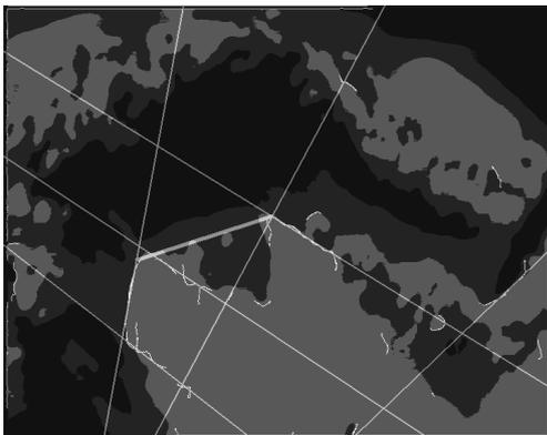
Figure 3: Finding the right direction of boundary combining perceptual grouping and colour-texture segmentation results.
