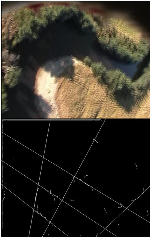
Figure 1: Our original frame of aerial video and extracted lines by the MSSE.
