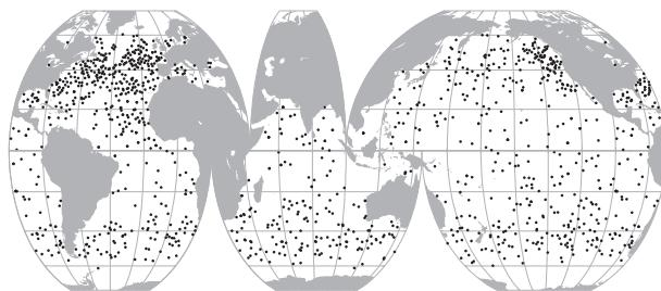
FIG. 6. Distribution of collocated measurements between *Jason-1* and *ERS-2* radar altimeters. During the latter part of the *ERS-2* mission, an onboard storage failure limited the spatial coverage to the Northern Hemisphere. As a result, there is a greater density of collocation points in the North Atlantic and parts of the North Pacific.
