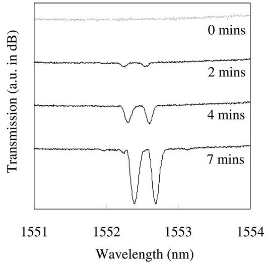
Fig. 2. Spectra near 1550 nm, showing the growth of a FBG in a 7 min exposure to 130 mW of CW UV laser light through a phase mask of periodicity 536 nm.
