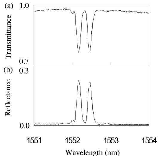
Fig. 3. Measured FBG (a) transmission and (b) corresponding reflection spectra at 1550 nm.
