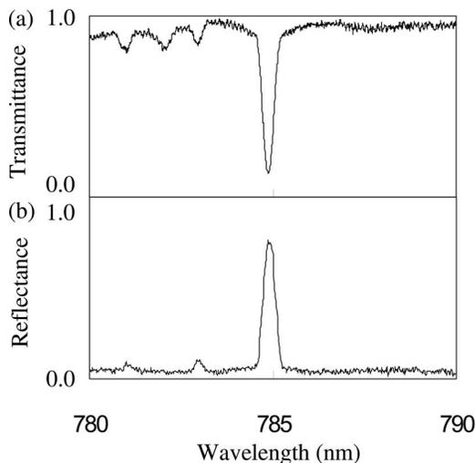
Fig. 1. Measured FBG (a) transmission and (b) corresponding reflection spectra at 785 nm.
