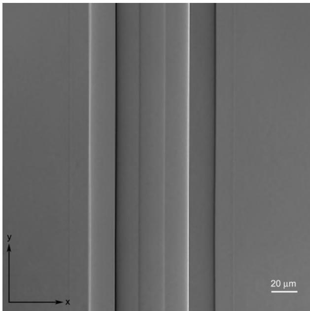
Fig. 1. Normalized DIC image of a CF2-082 multistep-index fiber covering an area of approximately  $1024 \times 1024$  pixels having a pixel spacing of approximately  $0.23 \mu\text{m}$ .
