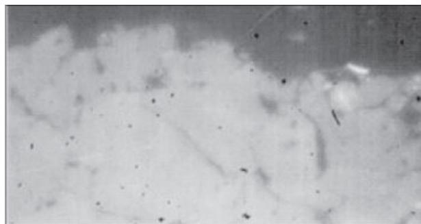
**Figure 3.** Cross section of a representative coating after erosion test. Cracks in the vertical (V) and parallel (P) direction are indicated.
