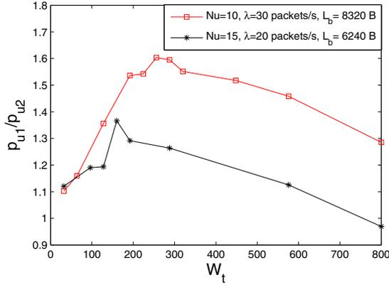
Fig. 3. The ratio of the collision probability of a small packet on its first attempt and retransmission attempts. (Scenario: an 802.11e EDCA WLAN with one greedy source sending large packets of  $L_b$  bytes,  $N_u$  quasi-periodic sources sending small packets of 100 bytes with rate of  $\lambda$ .)
