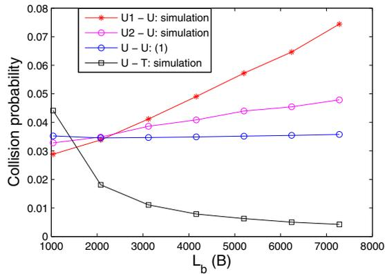
Fig. 2. The classification of the collision probability of a small packet. (Scenario: an 802.11e EDCA WLAN with one greedy source sending large packets of  $L_b$  bytes, 10 quasi-periodic sources sending small packets of 100 bytes with rate of 30 packets/s.)
