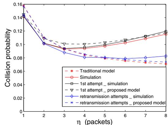
Fig. 4. Collision probability of a small packet from non-saturated sources. ( $N_u = 10$ ,  $N_t = 2$ ,  $\lambda = 30$  packets/s,  $l_{sat} = 1040$  bytes,  $l_{nonsat} = 100$  bytes,  $W_u = 32$ ,  $W_t = \eta W_u$ .)
