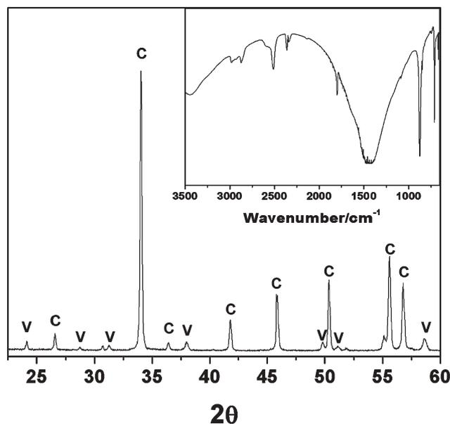
**Fig. 3** X-ray diffraction pattern and FTIR spectrum (inset) of calcium carbonate precipitates obtained after reaction in 0.5 M urea and 1 M CaCl<sub>2</sub> solution for 24 h. Samples were separated from the reaction solution and washed with water by centrifugation and dried overnight under vacuum. Peaks coded as C and V, respectively, are characteristic of calcite and vaterite.
