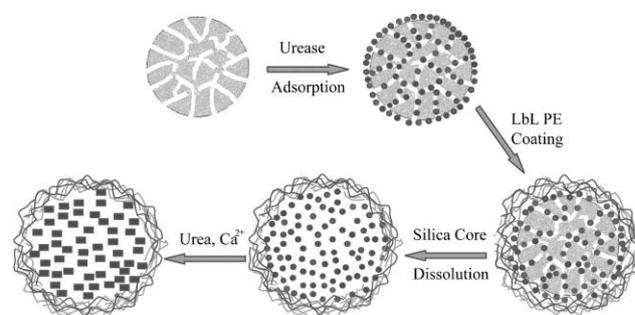
**Fig. 1** Schematic representation of the procedure for encapsulating urease in polypeptide microcapsules using MS spheres as templates and their use as biomimetic reactors to form CaCO<sub>3</sub> within the capsules.
