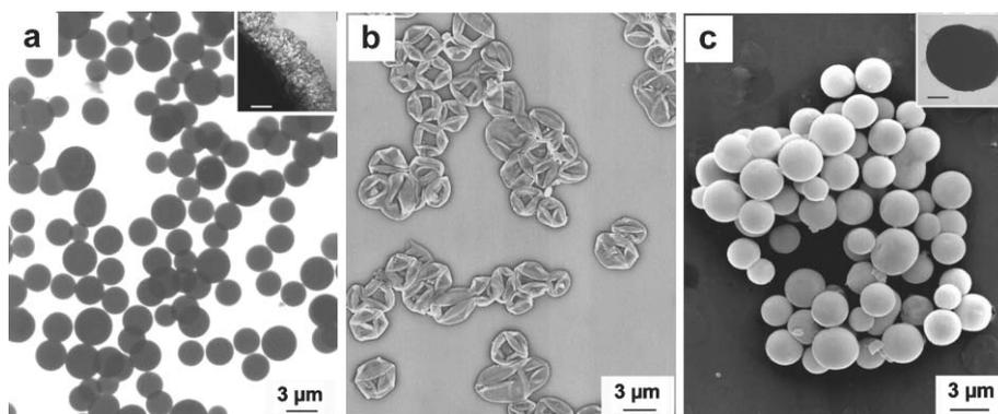
**Fig. 2** Low (a) and high magnification (a, inset, scale bar 100 nm) TEM images of MS spheres. SEM images of urease-loaded (PLL/PGA)<sub>3</sub> capsules before (b) and after (c) carbonate precipitation in 0.5 M urea and 1 M CaCl<sub>2</sub> solution for 20 min. Inset of image c: TEM image of urease-loaded (PLL/PGA)<sub>3</sub> capsules after carbonate precipitation for 20 min. Scale bar: 1 μm.
