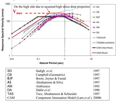
Fig. 3. Comparison of response spectra from different attenuation relationships (M7 R=30km on rock)
