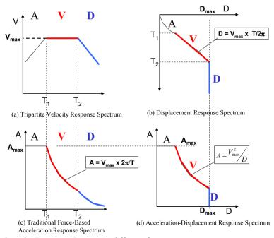
Fig. 1. Earthquake Response Spectra in different formats
