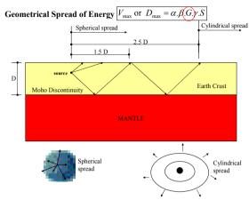
Fig. 7. Schematic representation of geometrical attenuation
