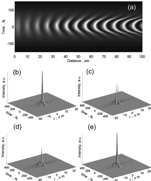
Fig. 1. (a) Calculated  $zt$  image of the on-axis pulse intensity in the moving coordinate frame. (b)–(e) Space-time-resolved energy fluence profiles of the wave packets at distances between  $z=50\ \mu\text{m}$  and  $z=58.5\ \mu\text{m}$ , representing the refocusing cycle of the GB beam in glass.
