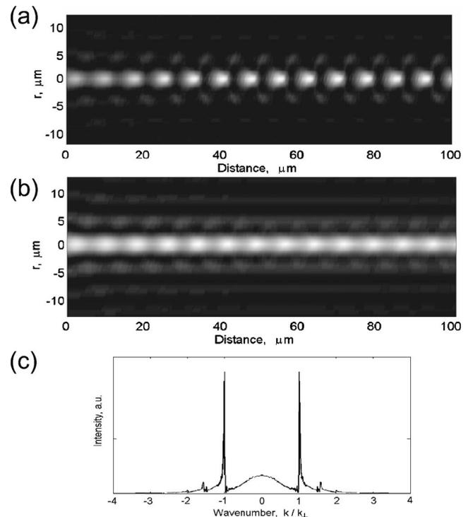
Fig. 2. (a) Instantaneous (at  $t=0$  in the moving coordinate frame) intensity, (b) fluence, and (c) the angular spectrum calculated for the GB wave packet propagating for  $100\ \mu\text{m}$  in glass.
