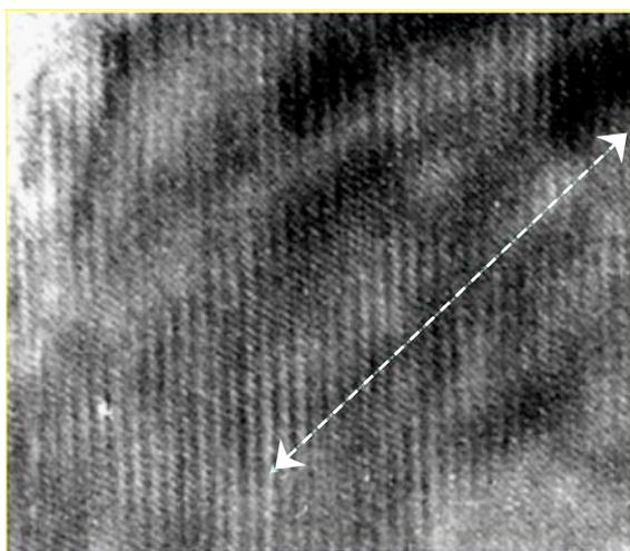
**Fig.1.** TEM image of the region analysed in Fig.2. The arrow marks the direction of the  $0.16$  nm periodicity.
