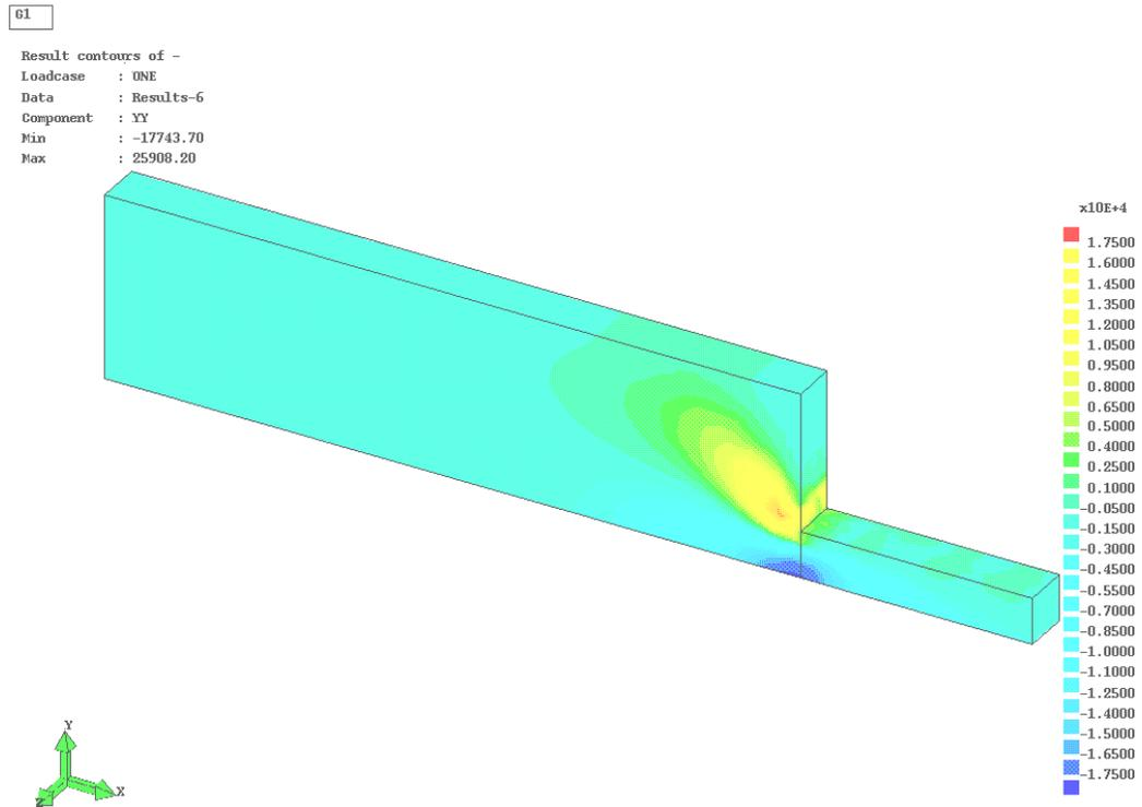
Figure 5.3-5. Stress contours for yy components in 4:1 planar contraction.
