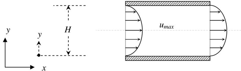
Figure 5.2-1. Steady laminar flow between horizontal Parallel Plate.
