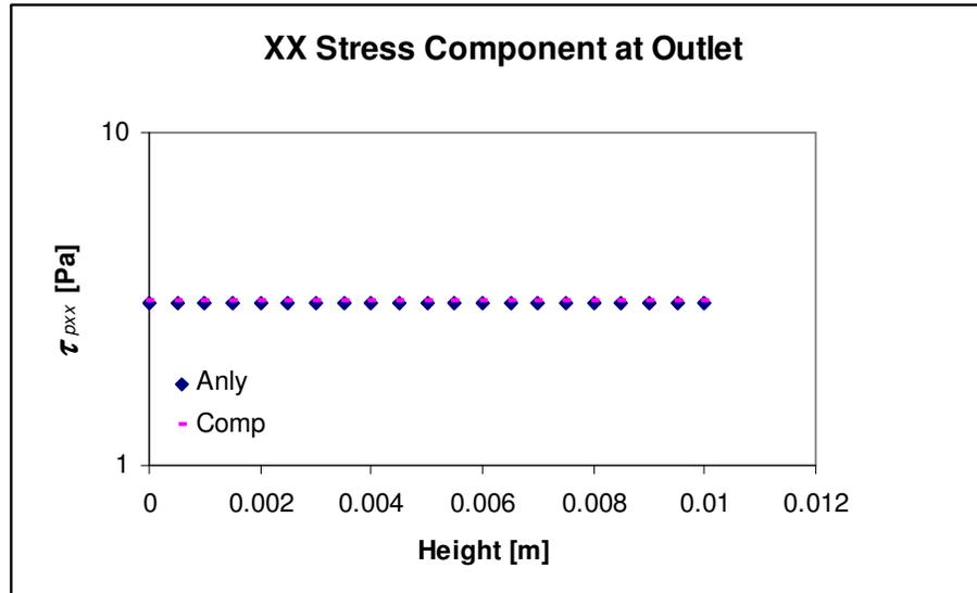
Figure 5.1-4. Computational and analytical  $xx$ -scomponent of polymeric stress contribution to extra stress tensor for simple shear flow at outlet.
