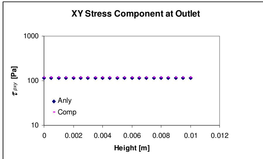
Figure 5.1-5. Computational and analytical  $xy$ -component of polymeric stress contribution to extra stress tensor for simple shear flow at outlet.
