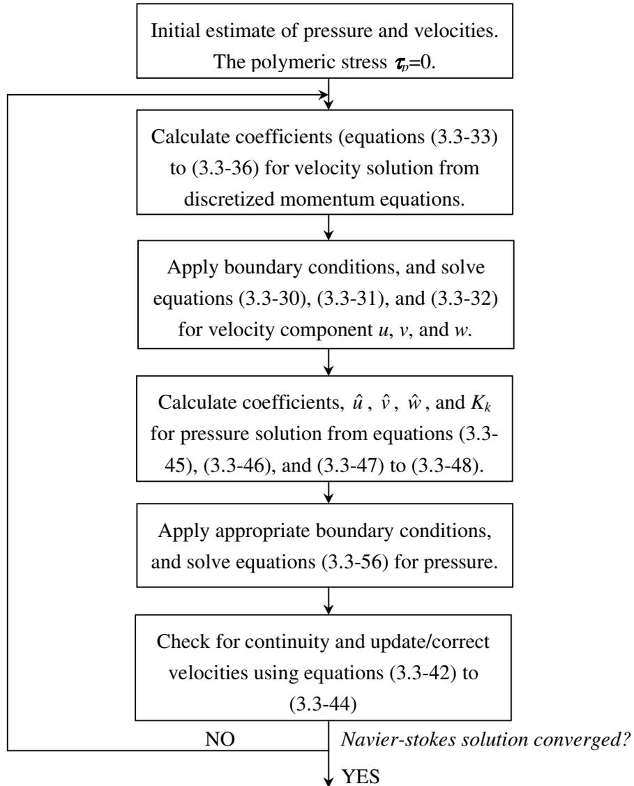
Figure 4.3-1. Solution schematic for Newtonian flow simulation.
