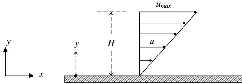
Figure 5.1-1. Simple shear flow.
