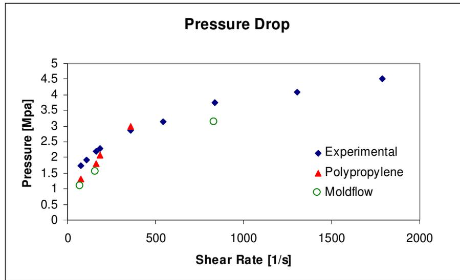
Figure 5.3-12. Comparison of experimental and computational pressure drop in 4:1 axisymmetric contraction.
