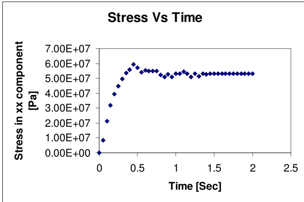
Figure 5.3-13. The  $xx$  stress component versus time at re-entrant corner in axisymmetric contraction.
