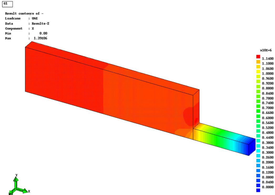
Figure 5.3-8. Pressure contours in 4:1 planar contraction.
