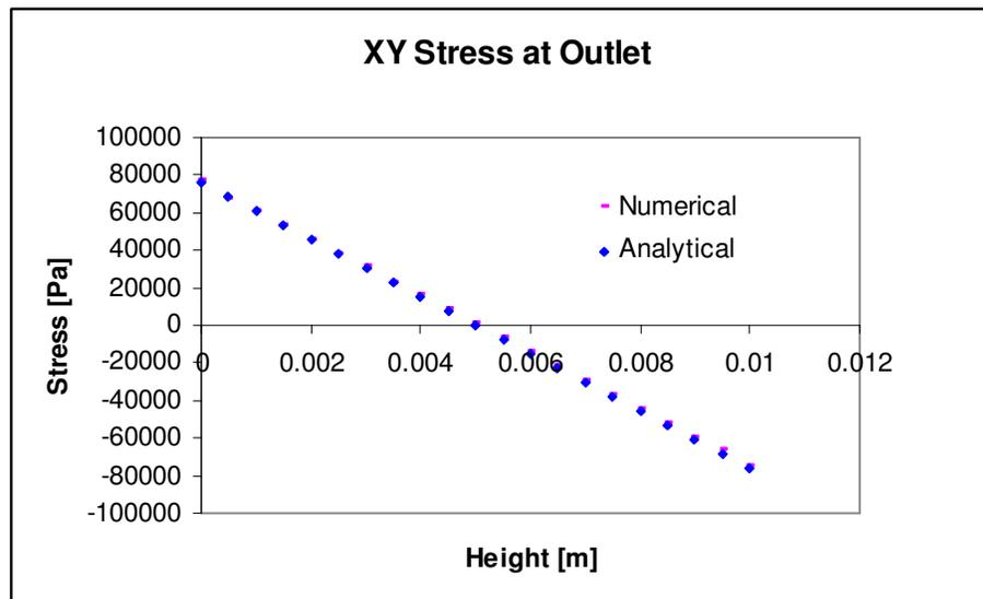
Figure 5.2-5. Computational and analytical  $xy$  component of polymeric stress contribution to extra stress tensor at the outlet for planar Poiseuille.
