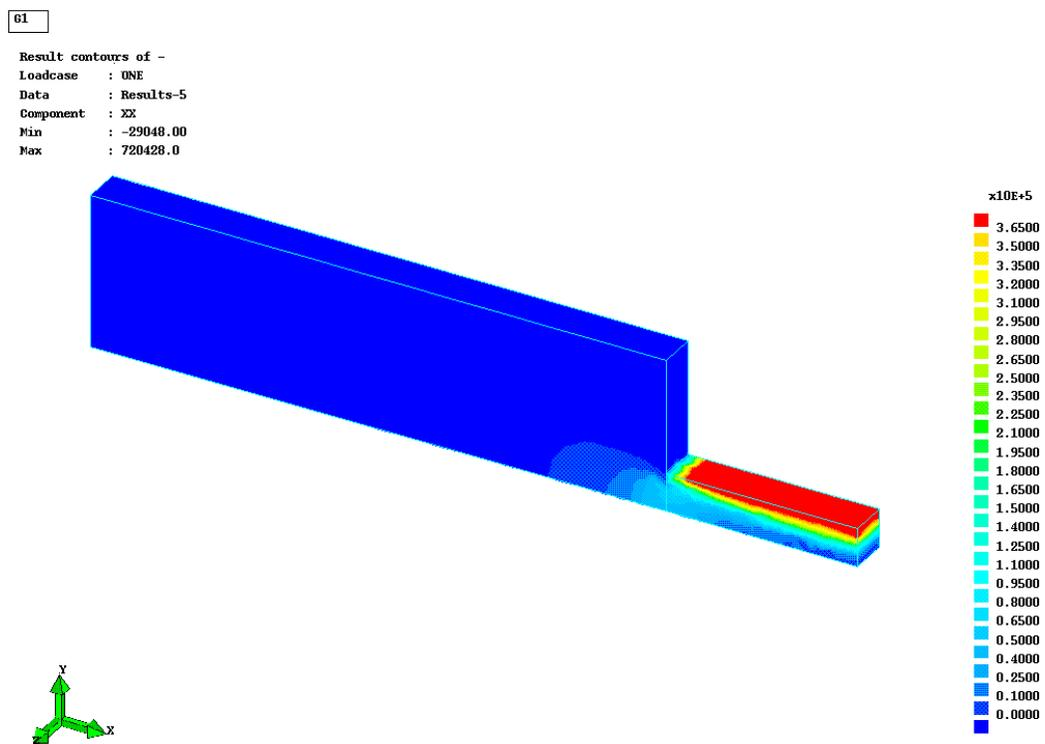
Figure 5.3-3. Stress contours for  $xx$  components in 4:1 planar contraction.
