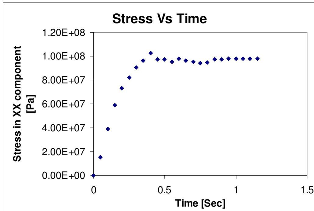
Figure 5.3-10. The  $xx$  stress component vs time at re-entrant corner in planar contraction.
