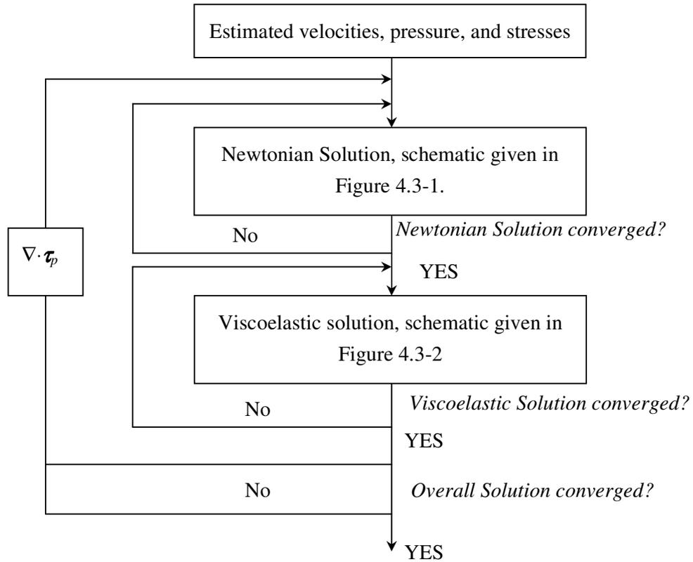
Figure 4.3-3. Overall solution schematic.
