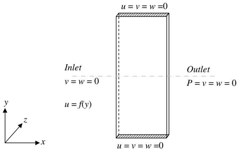
Figure 5.2-2. Velocity boundary conditions for horizontal parallel plate in laminar steady state flow.
