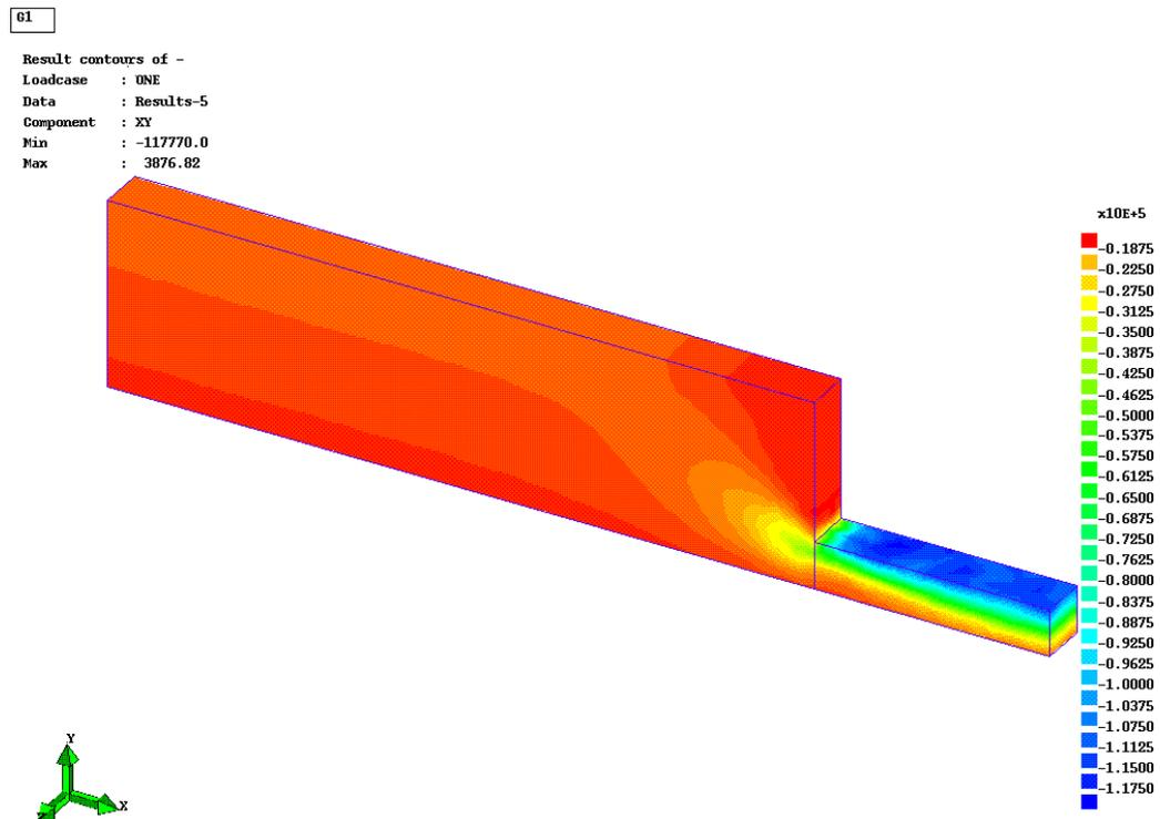
Figure 5.3-4. Stress contours for  $xy$  components in 4:1 planar contraction.
