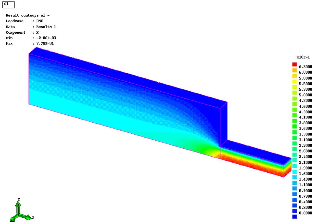
Figure 5.3-6. Velocity contours for  $x$  direction in 4:1 planar contraction.
