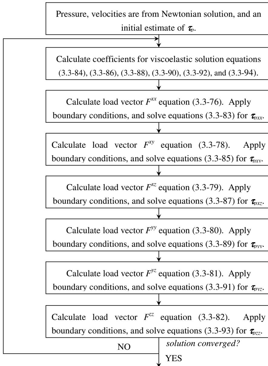
Figure 4.3-2. Solution schematic for Viscoelastic flow simulation.
