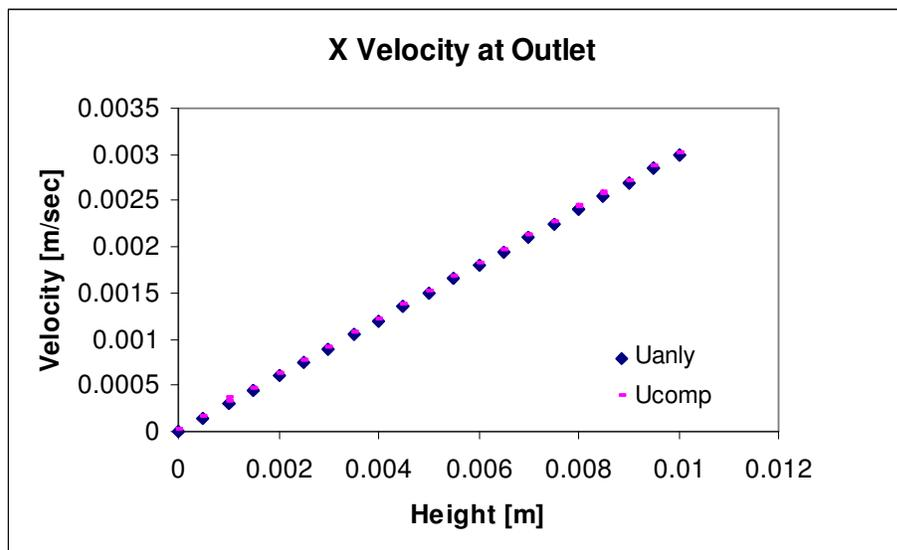
Figure 5.1-3. Computational and analytical  $x$ -velocity for simple shear flow at outlet.
