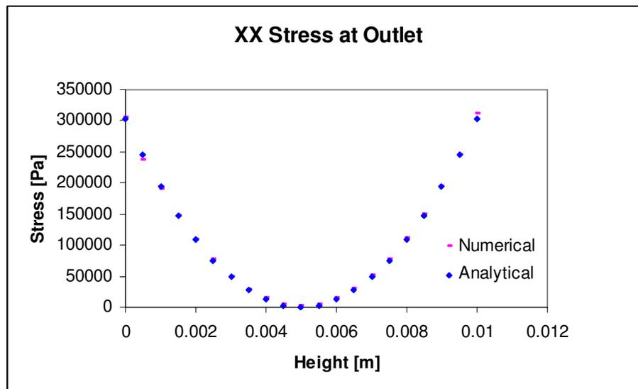
Figure 5.2-4. Computed and analytical  $xx$  component of polymeric stress contribution to extra stress tensor at the outlet for planar Poiseuille flow.
