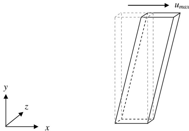
Figure 5.1-2. Flow in Simple Shear Geometry.
