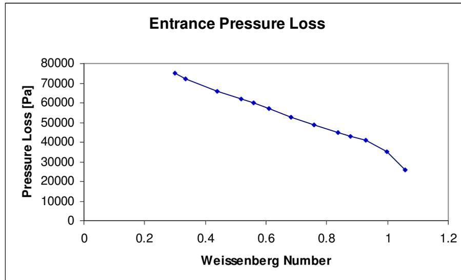
Figure 5.3-9. Entrance pressure loss for Oldroyd-B fluid in 4:1 planar contraction.
