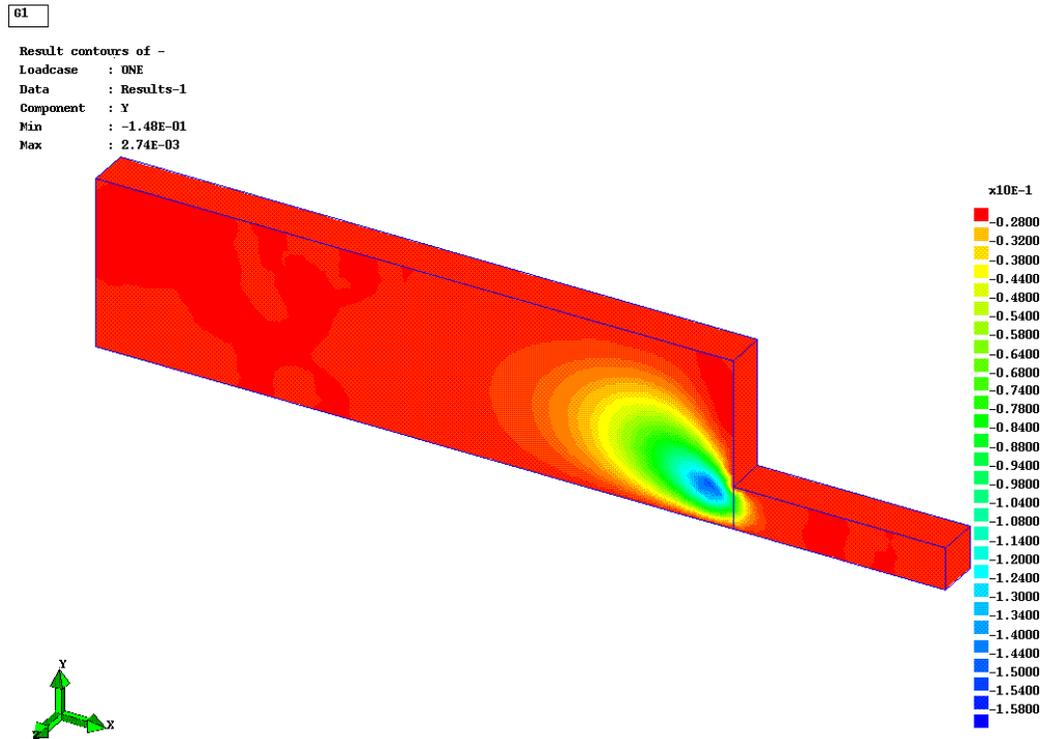
Figure 5.3-7. Velocity contours for y direction in 4:1 planar contraction.
