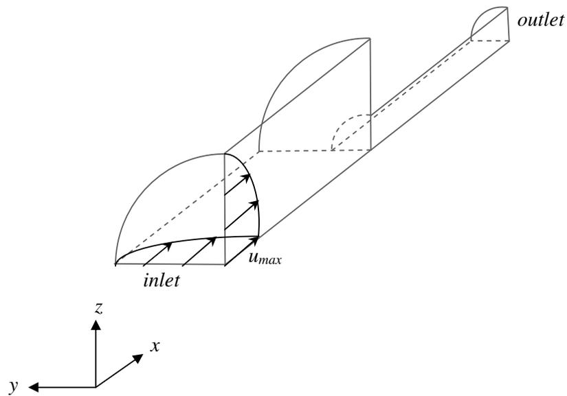
Figure 5.3-10. Velocity boundary conditions for axisymmetric 4:1 contraction.
