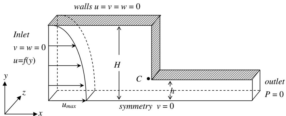
Figure 5.3.2. Velocity boundary conditions for 4:1 planar contraction.
