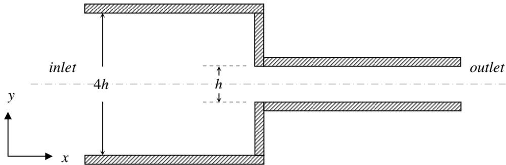
Figure 5.3-1. Schematics diagram of a 4:1 contraction problem.
