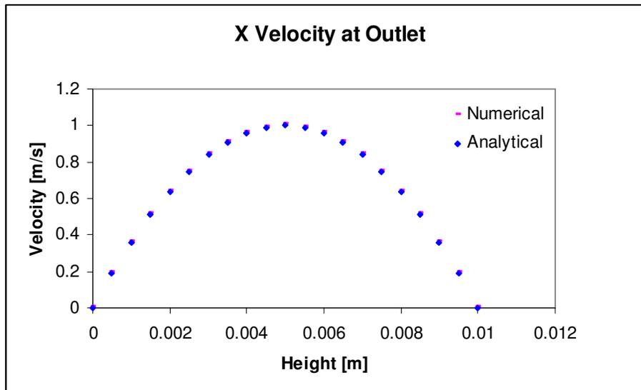
Figure 5.2-3. Computational and analytical  $x$ -velocity at outlet of horizontal parallel plate arrangement.
