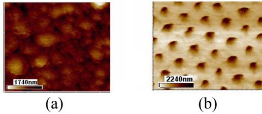
Figure 1. Typical 2D AFM images of the as-received (a) and modified (b) fibre substrates (scanned areas  $4 \mu\text{m} \times 4 \mu\text{m}$ ).
