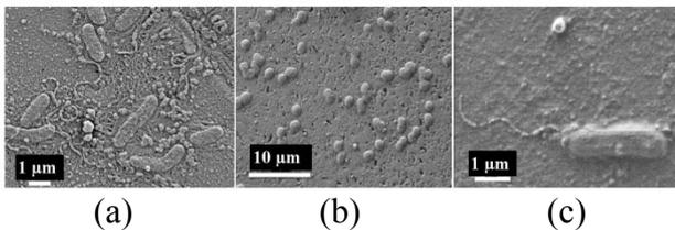
Figure 2. Typical SEM image of *P. issachenkonii* (a), *C. marina* (b) and *P. aeruginosa* (c) cells and EPS deposits on the as-received fibre surface.
