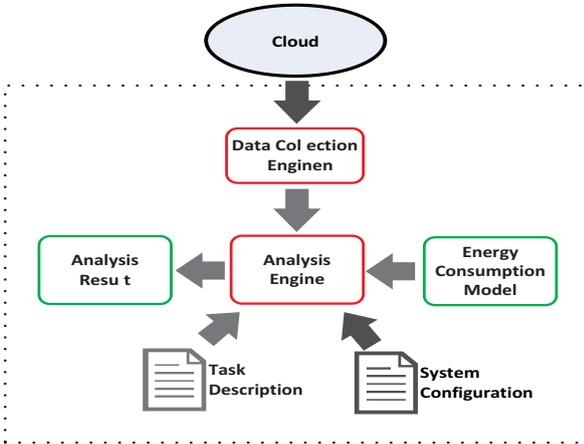
Figure 1. Architecture of our energy consumption analysis tool.
