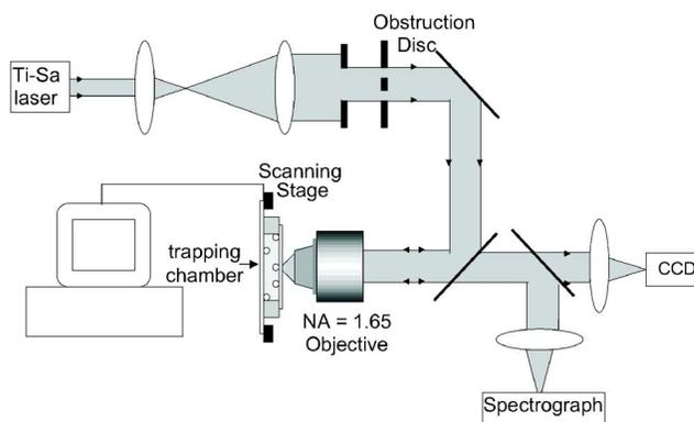
FIG. 1. (Color online) The schematic diagram of the experimental setup used to perform focused evanescent trapping using a pulsed laser.
