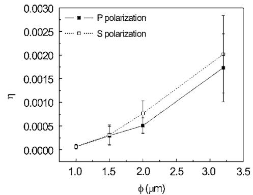
FIG. 3. Maximum near-field trapping efficiency  $\eta$  as a function of the particle diameter  $\phi$  for femtosecond laser illumination ( $\lambda=780$  nm,  $\varepsilon=0.86$ ).
