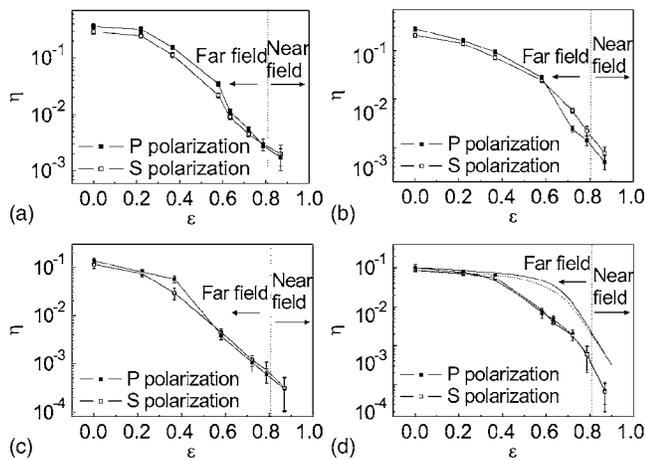
FIG. 2. The logarithmic values of the maximum transverse trapping efficiency  $\eta$  measured as a function of  $\varepsilon$  for femtosecond laser trapping ( $\lambda=780$  nm), for (a)  $\phi=3.2$   $\mu\text{m}$ , (b)  $\phi=2$   $\mu\text{m}$ , (c)  $\phi=1.5$   $\mu\text{m}$ , and (d)  $\phi=1$   $\mu\text{m}$ . (d) Shows the theoretical plot of trapping efficiency values computed using vectorial model.
