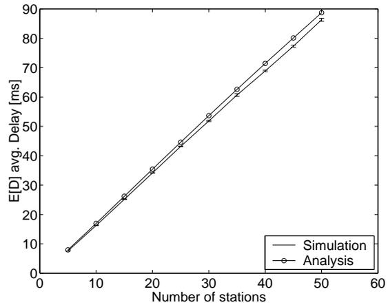
**Fig. 2.** Average access delay, UDP payload of 1000 bytes.
