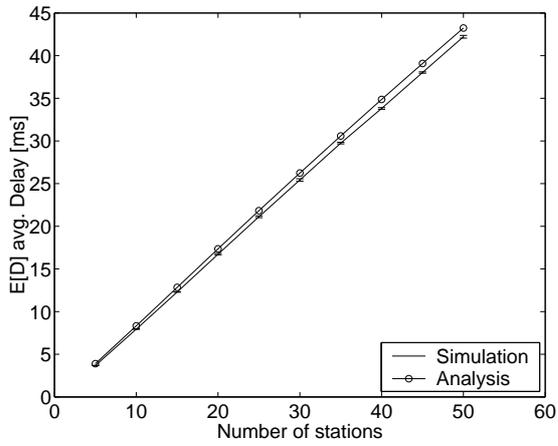
**Fig. 1.** Average access delay, UDP payload of 33 bytes.
