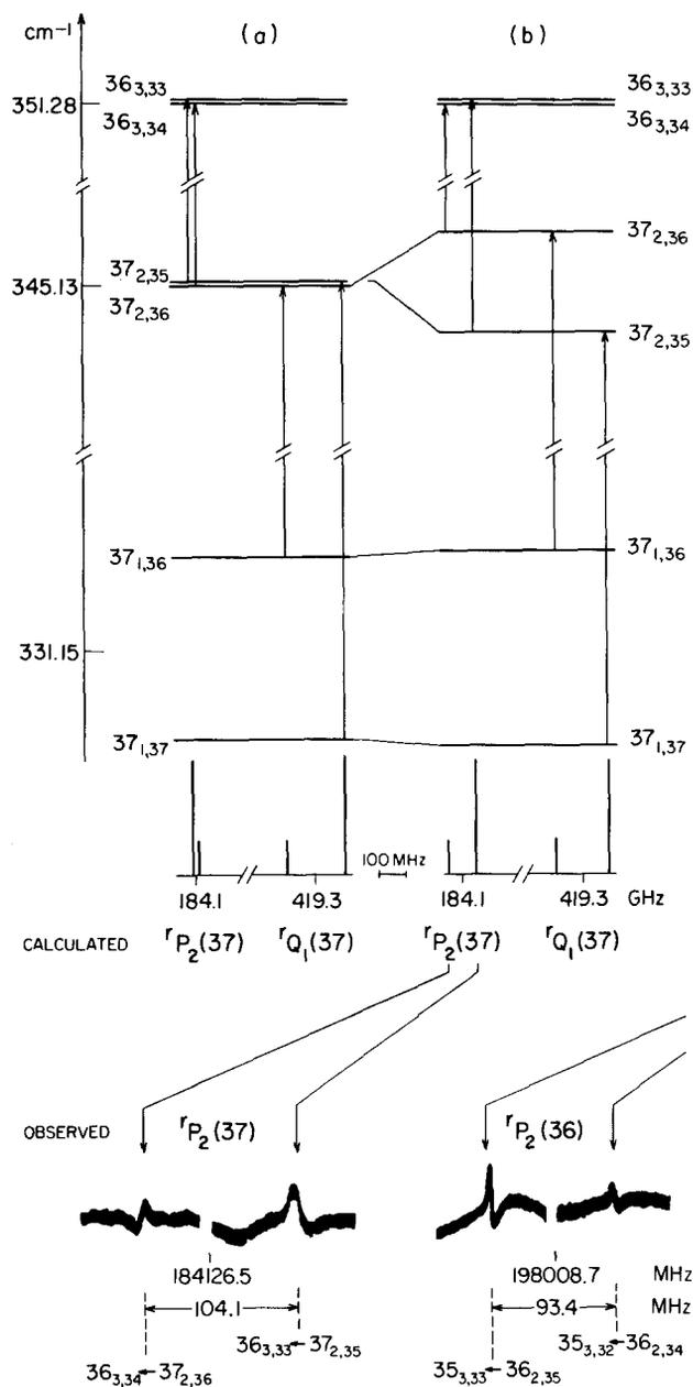
FIG. 1. Energy diagram for the  $\nu P_2(37)$  and  $\nu Q_1(37)$  transitions. The calculated intensity pattern of the  $\nu P_2(37)$  doublet may be compared with the observed transitions  $\nu P_2(37)$  and  $\nu P_2(36)$ .  $\nu Q_1$  transitions are reported in Ref. 3.
