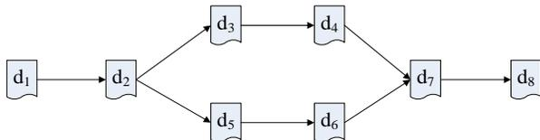
Figure 2. A simple Data Dependency Graph (DDG)
