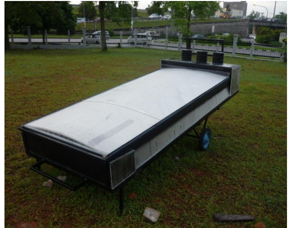
Figure 4.7b: Internal condensation condition under a wet morning (0.2m chimney)
