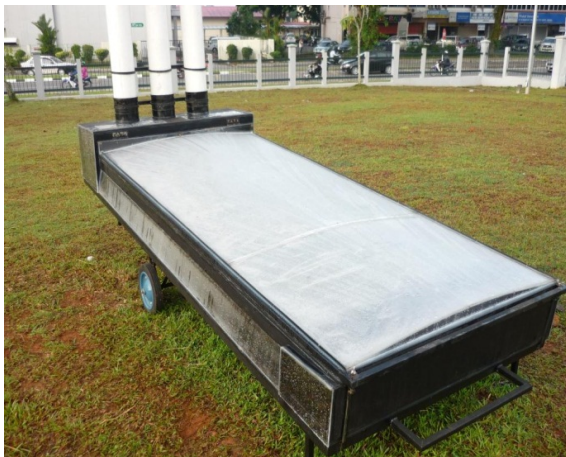
Figure 4.7c: Internal condensation condition under continuous rainy days – a view on a wet morning (1.5m chimney)
