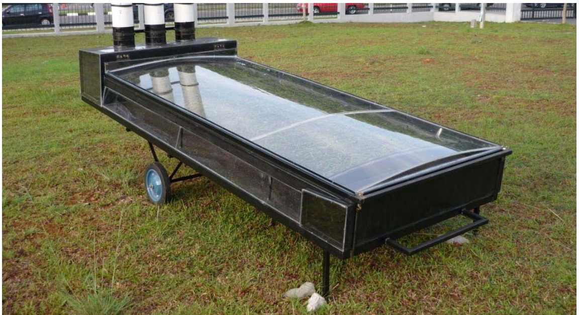
Figure 4.4: The dryer operates in a sunny day - picture taken during low sunlight moment to reduce reflection
