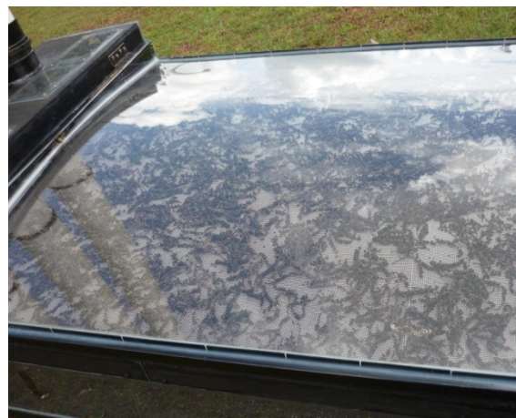
Figure 4.5d: A partial view to the drying tray at the early afternoon (1pm) on the second day. The pepper is left until 3pm under cloudy afternoon (2m chimney setting)
