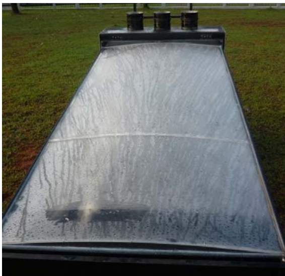
Figure 4.8: The water path showing at the inner side of the acrylic covers caused by the droplets drifted as the cover was opened – a view on a wet morning (0.2m chimney)
