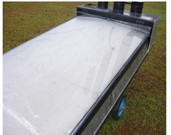
Figure 4.7d: Internal condensation condition under continuous rainy days – a view on a wet morning (2.0m chimney)
