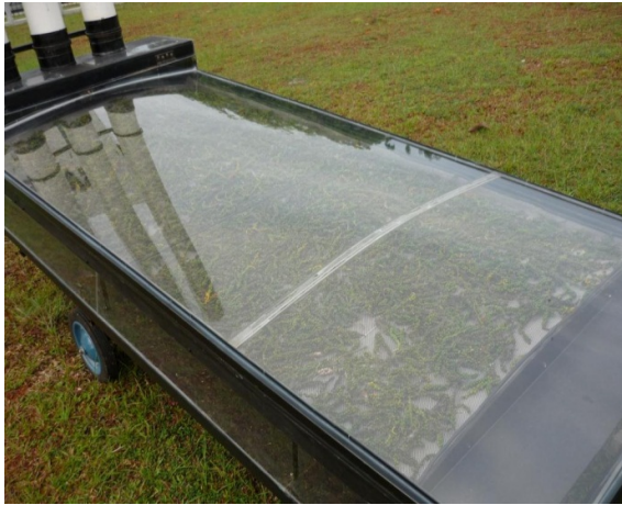
Figure 4.7a: Internal condensation condition under a dry morning (2.0m chimney)
