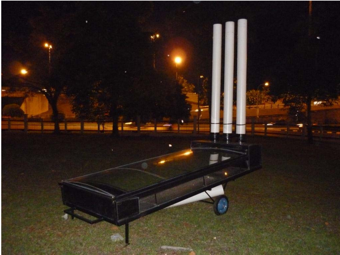
Figure 3.9a: The actual view of the proposed mixed-mode solar tunnel dryer that utilises varies chimney length to control the internal climate
