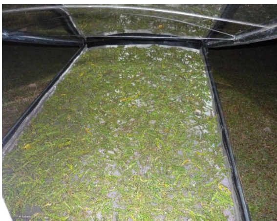
Figure 4.5a: A view to the drying tray during the first evening (fresh spikes) in a fine evening after a hot sunny day (2m chimney setting)
