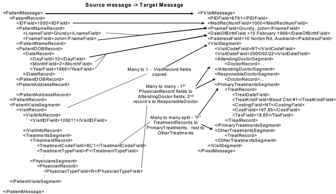
Figure 1. Illustration of mappings between XML formats
