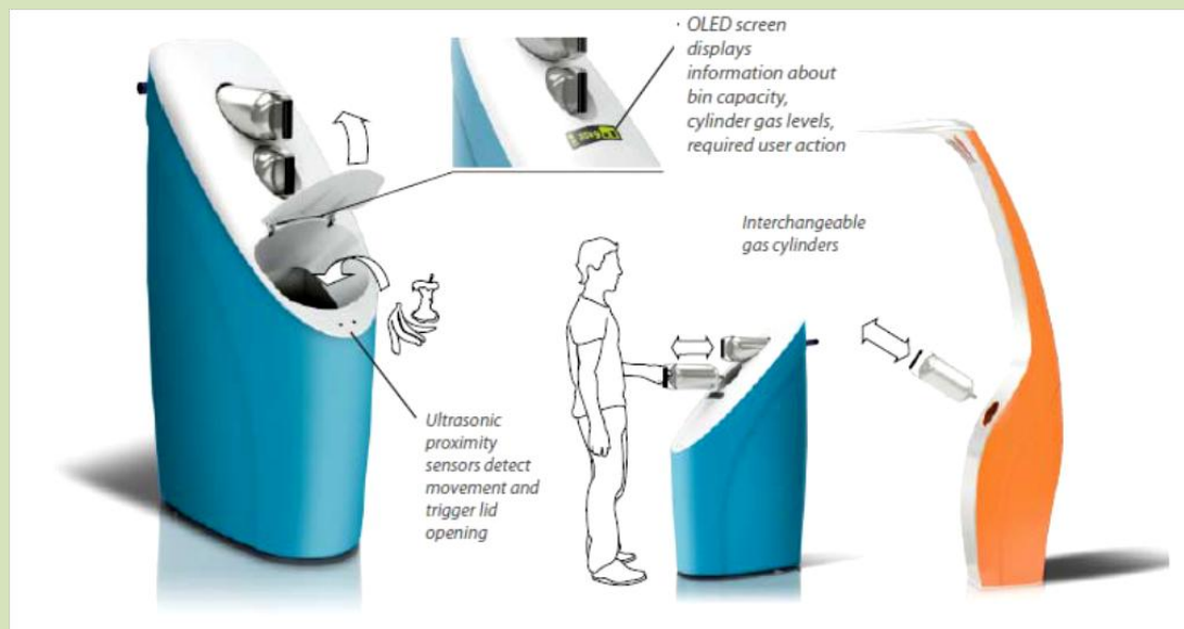
Figure Cs1.10: 2012 EDF Sustainable Design Challenge winner Gastrom biogas generator converts restaurant food scraps to methane through anaerobic digestion. (Image source: final year PDE students)
