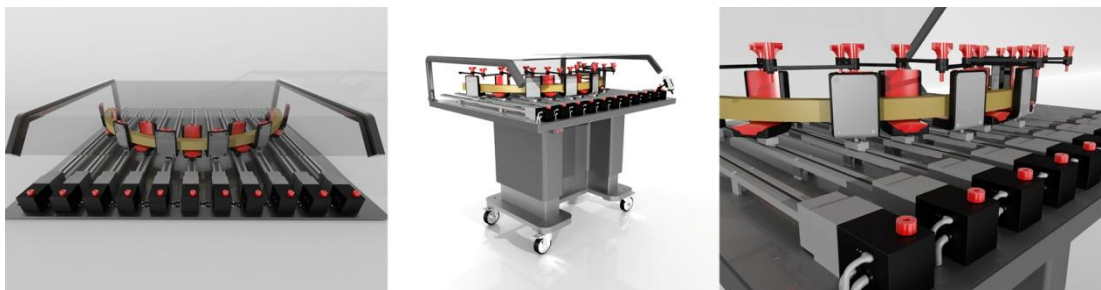
Figure 5.1: Wood forming equipment using linear actuators to retain the shape during the drying process –a collaborative research and design project (image source: final year Swinburne Product Design Engineering student)
