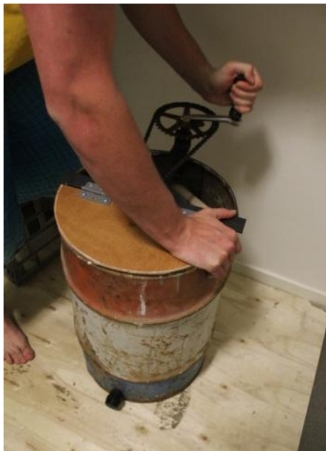
Figure 1.8: Examples of socially responsible design – a honey extractor made from readily accessible materials for remote Ugandan communities by Swinburne PDE student (left) and solar lantern for developing nations by Glasgow School of Art PDE student (right) (image source: student designs)
