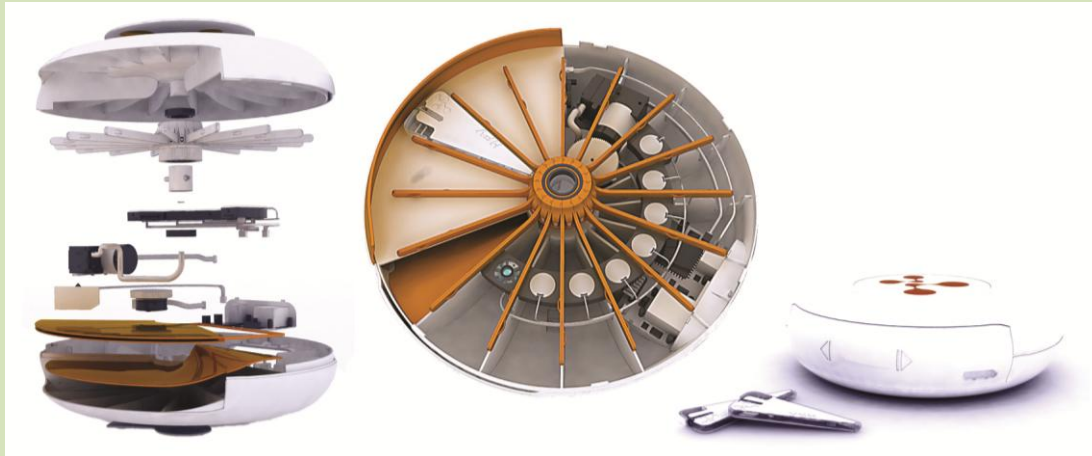
Figure Cs1.3: Medical diagnostics device utilising microfluidics technology to detect HPV cervical cancer (Image source: final year Product Design Engineering project)
