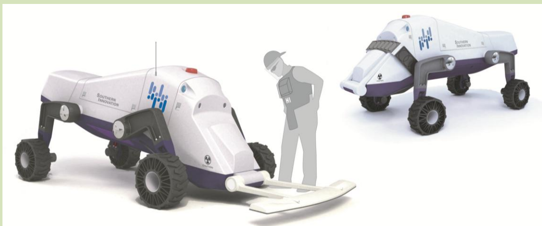
Figure Cs1.2: Landmine detection vehicle. A remote controlled self-levelling rugged terrain vehicle that uses gamma and metal detection systems to detect landmines without risk to personnel. (Image source: final year Product Design Engineering project)
