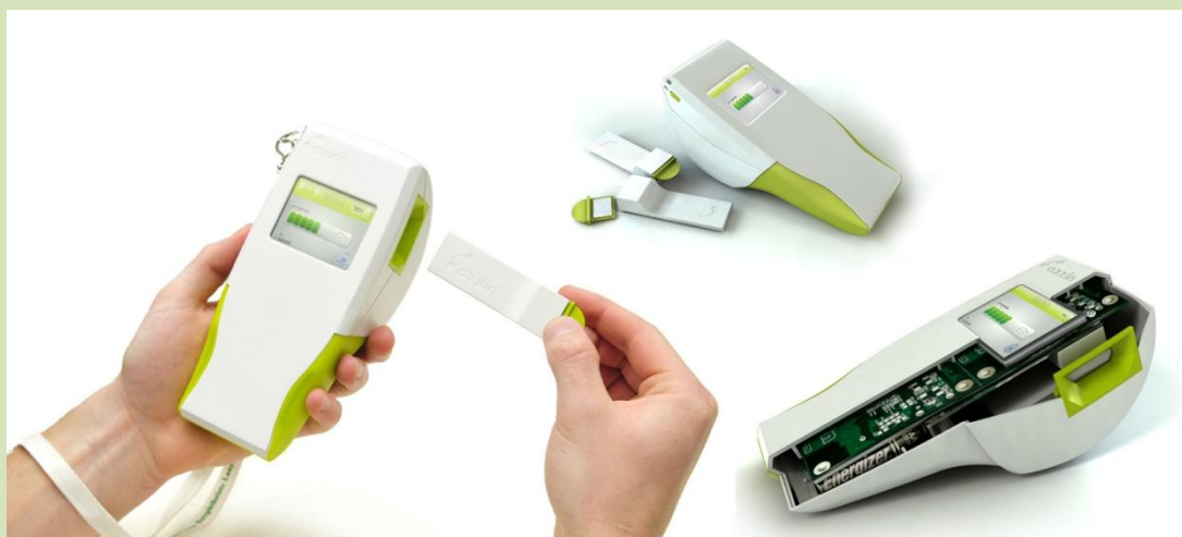
Figure Cs3.8: Design against crime - Roadside drug testing analysis unit for use by police (Image source: student design with industry partner- final year Product Design Engineering project)
