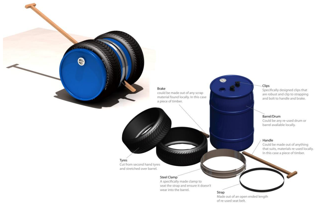
Figure 6.5: Product Design Engineering student outcome no.1 - an innovative solution that utilises readily available found objects (Image source: PDE student design - final year open-ended project)
