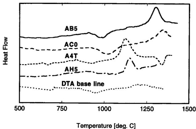
Fig. 4 Results of the differential thermal analysis (DTA) measurements
