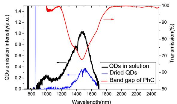
Figure 1. (left) Excitation spectrum of self-made PbSe QDs in solution (black line) and dried QDs on cover slip (blue line). (right) Band gap of 3D woodpile PhC (red line, after baseline).
