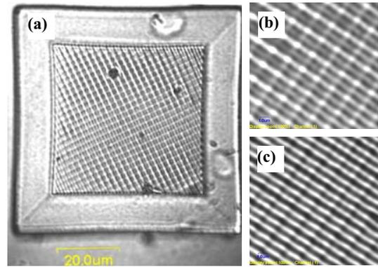
Figure 4. Microscopy images of 3D woodpile PhC fabricated with QDs doped composite. (a) Overall image; (b) Image of cross layers; (c) Image of single layer. Lattice constant:  $1 \mu\text{m}$ ; Size:  $50 \times 50 \times 14 \mu\text{m}$ .
