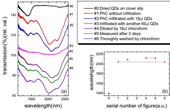
Figure 2. (a) Baseline transmission spectra of QDs and PhC under different processes; (b) Centre wavelength of the photonic band gap in (a). From #0 to #6, the wavelength is 1396, 2045, 2093, none, 2125, 2118, 2040 nm, respectively. From #4 to #5, the spectrum remained unchanged for three days, which showed the repeatable measurements and the stability of infiltrated structures.
