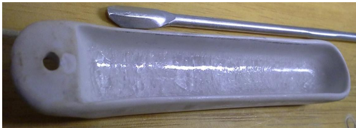
Figure 6.7.3: The binary salt two minutes after brought out from HT furnace. Within a short period, the salt surface started to crystallize.
