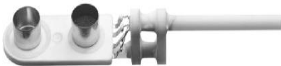
Figure C.2.4 (b): Horizontal DSC/TGA ceramic transducer for sample temperature and heat flow measurement [414].
