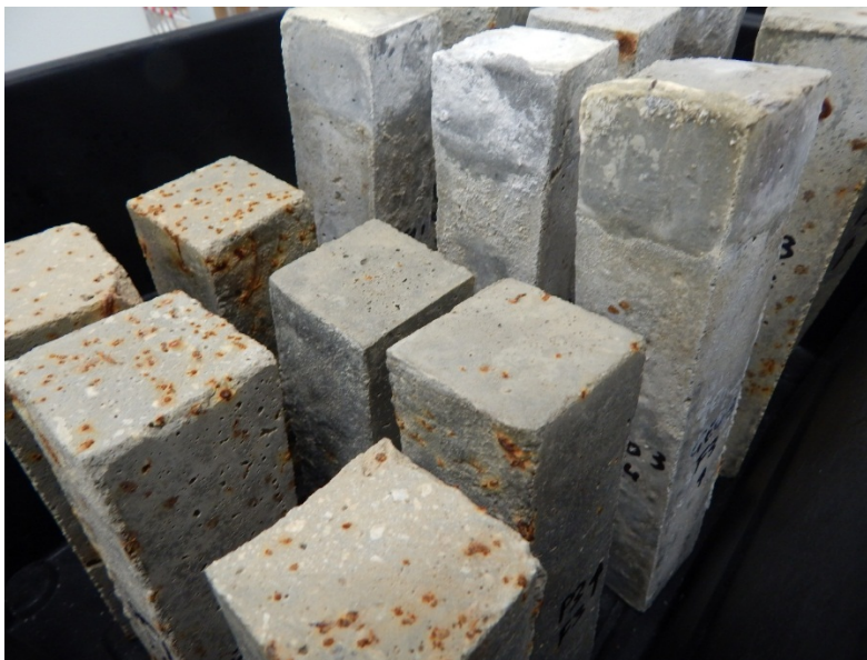
Figure 4. 1: The 15 test prisms immersed in aerated seawater for 6 months shown after removal from the tank at the end of the experiment
