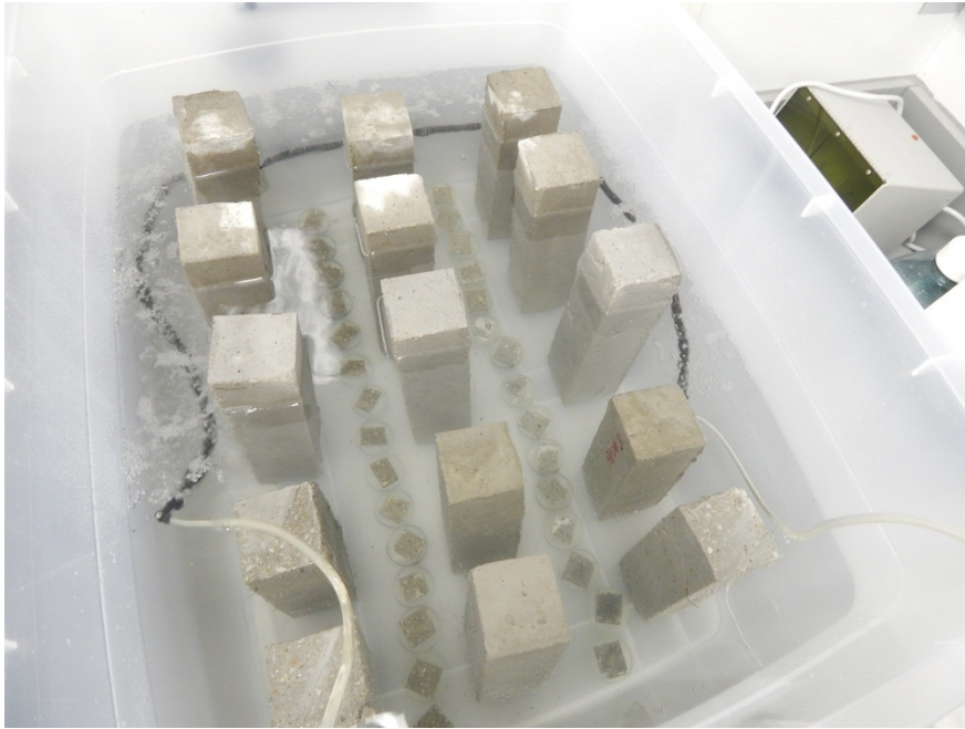
Figure 2. 7: Experimental setup used for immersion of the steel fibre reinforced mortar samples in aerated seawater.
