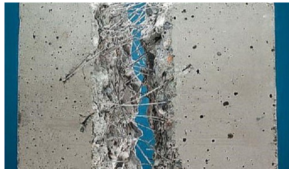
Figure 1. 2: Typical distribution of steel fibres when concrete fractures (ACI)
