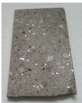
Figure 2. 10: Typical cross-section used for fibre count. The shiny steel fibres are clearly visible in the mortar.
