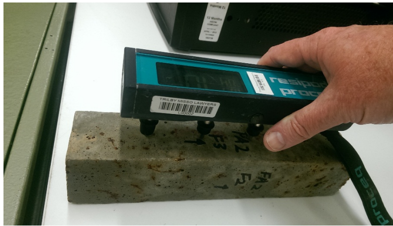
Figure 2. 8: The Proceq probe used to take electrical resistivity readings on a typical steel fibre reinforced mortar prism
