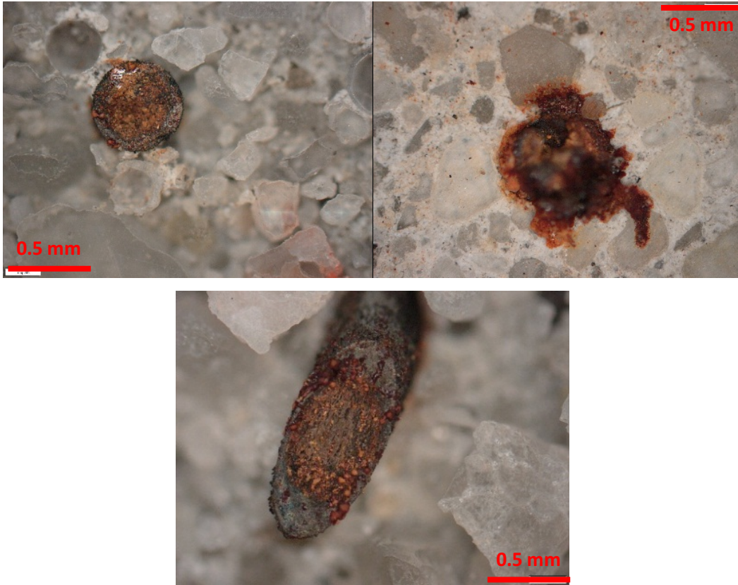
Figure 3. 17: Fibres in the OPC (left) and FA (centre and right) matrix after 4 months of immersion
