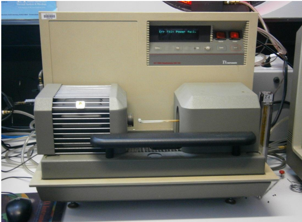
Figure 3-16: Conditioned of samples in thermogravimetric (TGA) chamber
