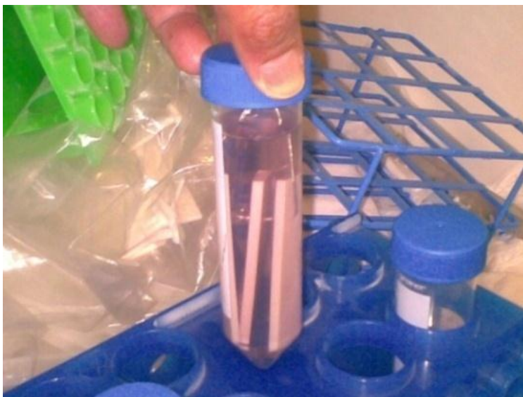
Figure 3-6: Immersion of PLA samples in a covered tube
