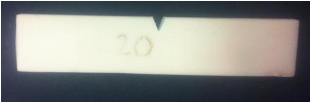
Figure 3-11: The notched samples for impact testing
