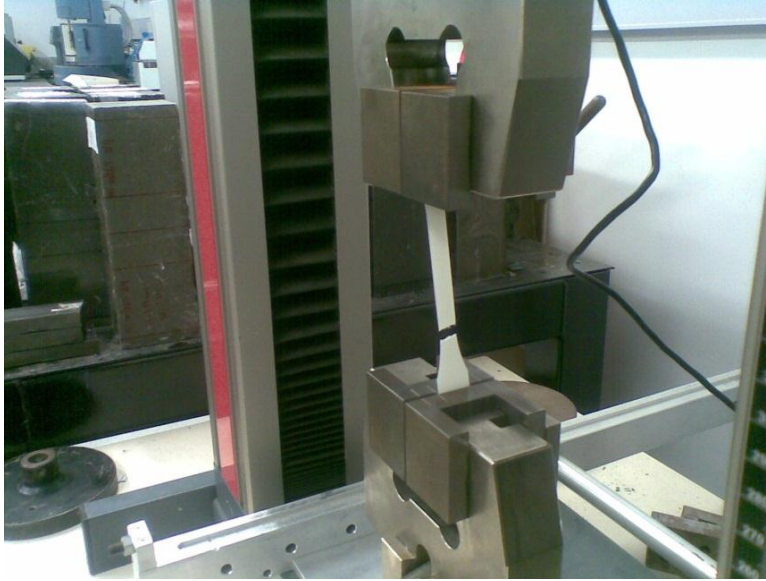
Figure 3-8: Break of tested sample held by a twin-self clamping jaw after load applied in tensile test
