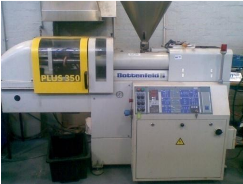
Figure 3-3: Battenfeld BA 350/75 injection moulding machine
