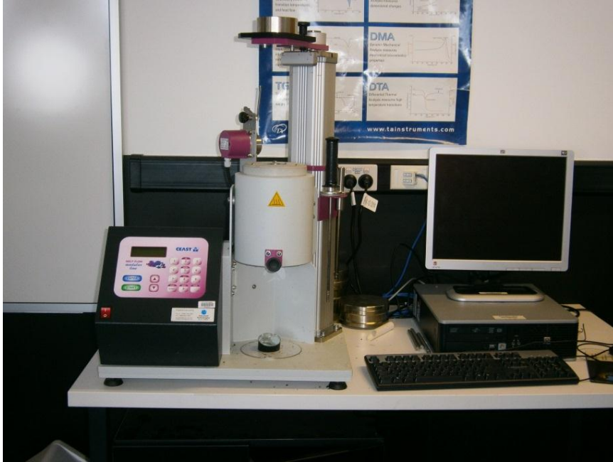
Figure 3-2: Melt flow rate measurement in CEAST instrument
