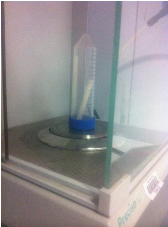
Figure 3-7: Weight measurement of an immersed sample in closed weighting bottle using analytical balance
