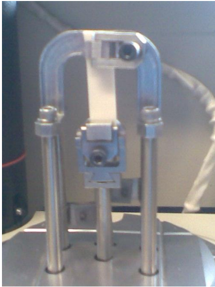
Figure 3-14: The tension film clamp of the TA Instruments DMA 2980
