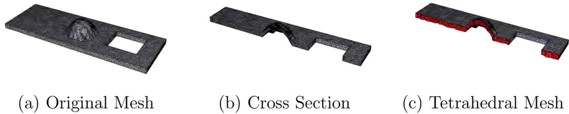
FIGURE 5.5: Tetrahedral mesh, shown in red, generated to preserve the volume of the mesh during the ACAP deformation.
