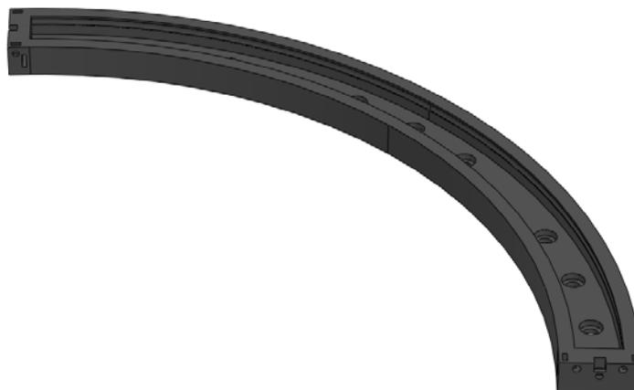
The radius of the rail is 150mm, this was chosen due to the minimum focal distance of the cameras, this distance could be reduced by using macro lenses , however, it is sufficient for the
