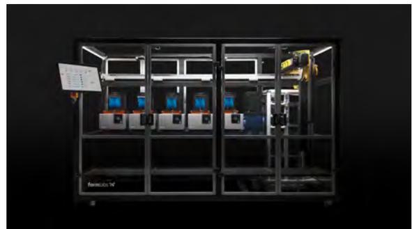
FIGURE 1.35: The Formlabs Form Cell, an automated approach to SLA 3D printing Formlabs (2017b).
