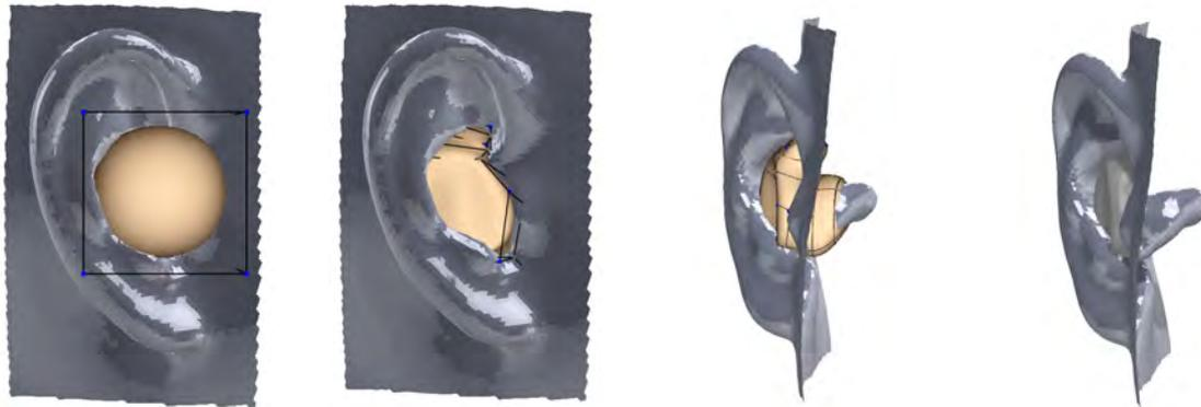
(a) Initialize Sub-D. (b) Drag to fit shape. (c) Slight over-size. (d) Cut using SSM.
