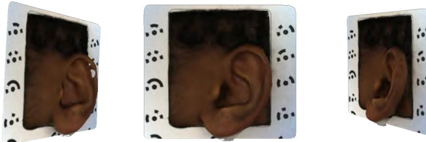
As can be seen in Figure 3.22, the algorithms were able to accurately reconstruct the dark complexion of this subjects ear. There is some noise and minor holes in the data, which could be due to issues with the image acquisition. During the process the participant had their ear placed very close to the grid which may have caused issues in the alignment process. However, the overall reconstruction is successful and has the majority of the desired information such as the inner ear region.
