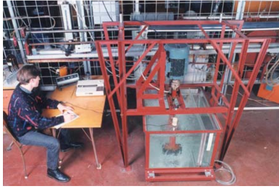
Figure 2. Full-scale model of a molten aluminium treatment furnace for the study of mixing, flow pattern and bubble dispersion.
