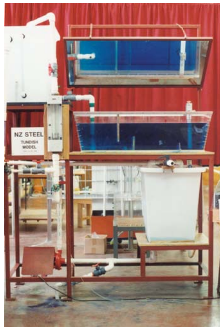
Figure 4. A One-third scale model of a tundish for the study of steel flow, mixing and residence time distribution.
