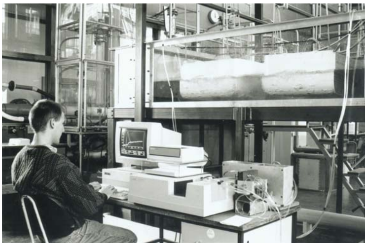
Figure 1. A full-scale aluminium smelting cell model used for the study of bubble-induced fluid circulation and mixing, side wall heat transfer, etc.
