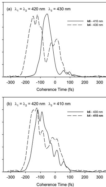
Figure 4. Time evolution of signal intensity taken from Fig. 3 at the four-wave mixing wavelength and the probe wavelength (in the  $\mathbf{k}_6$  direction).
