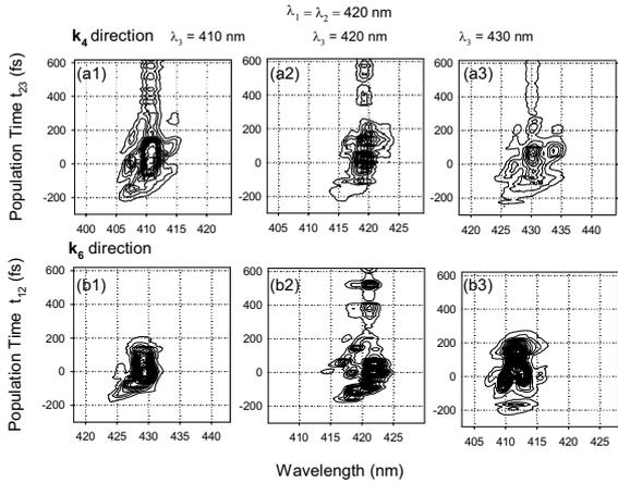
Figure 1. Time evolution of nonlinear signal spectra for 2  $\mu\text{m}$  undoped GaN epitaxial layer detected in the  $\mathbf{k}_4$  and  $\mathbf{k}_6$  directions versus population time  $t_{23}$  ( $t_{12}$ ) at various third-pulse wavelengths ( $\lambda_3$ ) and fixed coherence time  $t_{12} = 0$ .
