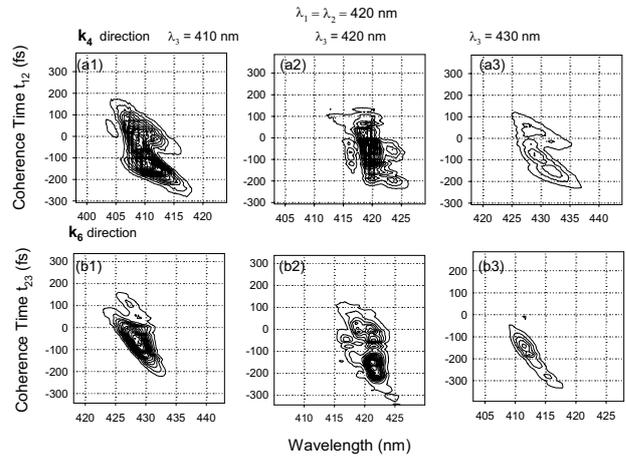
Figure 3. Time evolution of the nonlinear signal spectra from 2  $\mu\text{m}$  undoped GaN epitaxial layer detected in the  $\mathbf{k}_4$  (and  $\mathbf{k}_6$ ) directions versus coherence time  $t_{12}$  ( $t_{23}$ ) at various third-pulse wavelengths ( $\lambda_3$ ) and fixed population time  $t_{23} = -150$  fs (or  $t_{12} = -150$  fs).
