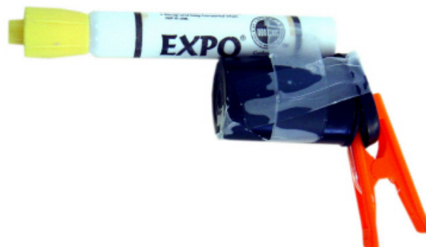
Figure 1. 3D sketch using ready-mades for a surgical instrument for Gyrus ENT by IDEO, 2008
