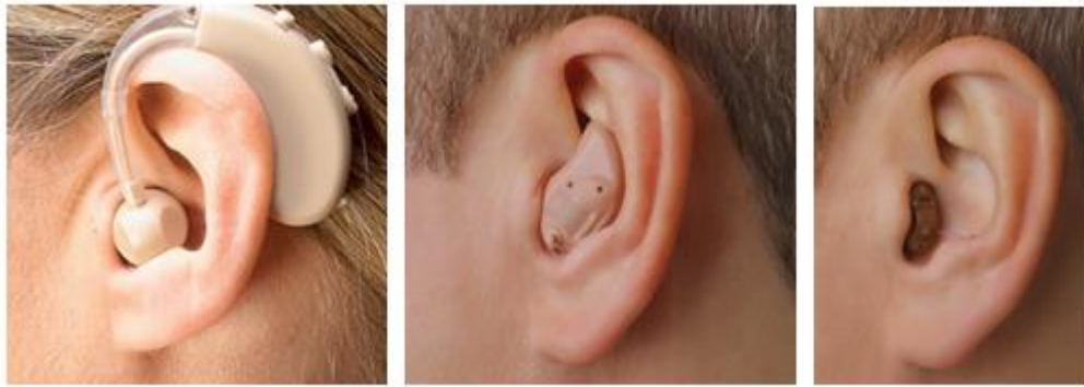
Figure 1.3 Examples of the three major types of currently available hearing aids - Behind-the Ear Hearing Aid, In-the-Ear Hearing Aid, and a Completely-In-the-Canal Hearing Aid (from left-to-right)
