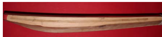
Figure 1(b). Cricket bat blade with an edge oak insert.
