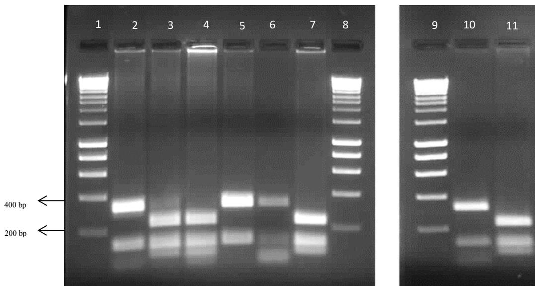
**Figure 3.3. Example of BsrB1 digested PCR products of *Pinb***
