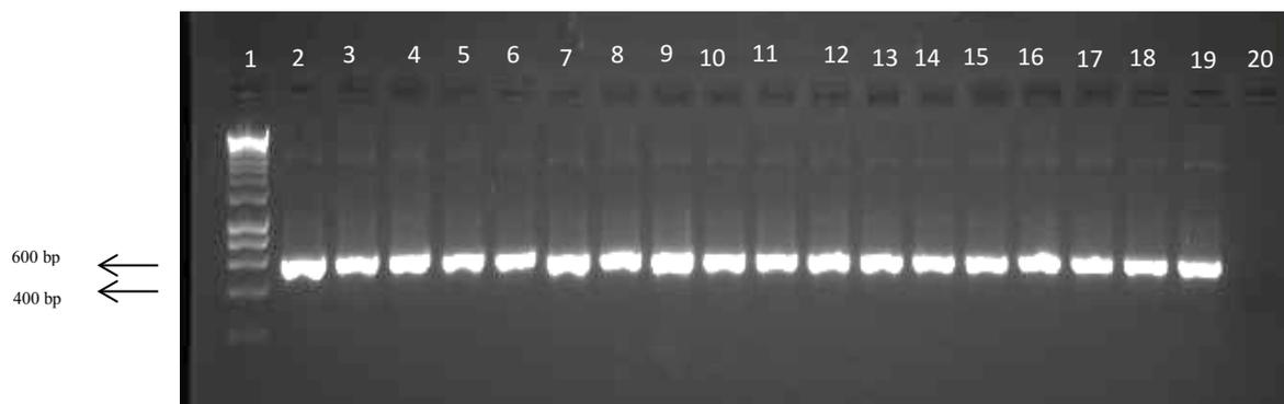
**Figure 3.11. Example of PCR products (using T7, SP6 primers) to screen for *Pinb-2* inserts.** Lane 1: Hyperladder1, lanes 2-19: amplified inserts from plasmids containing *Pinb-2* clones, lane 20: negative control (no template).
