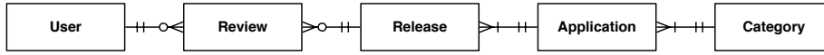
Figure 1: The cardinality of a Review, left by a User, per Release of an App in a Category.
