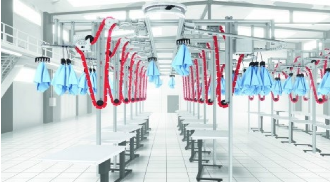
Figure 19 RFID Enabled automate operations (ETON 5000 syncro production system)
