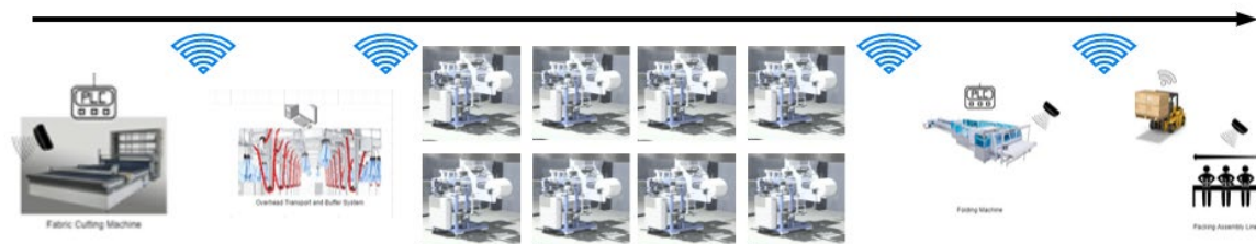
Figure 49 Mattress protector production flow and communication overview
