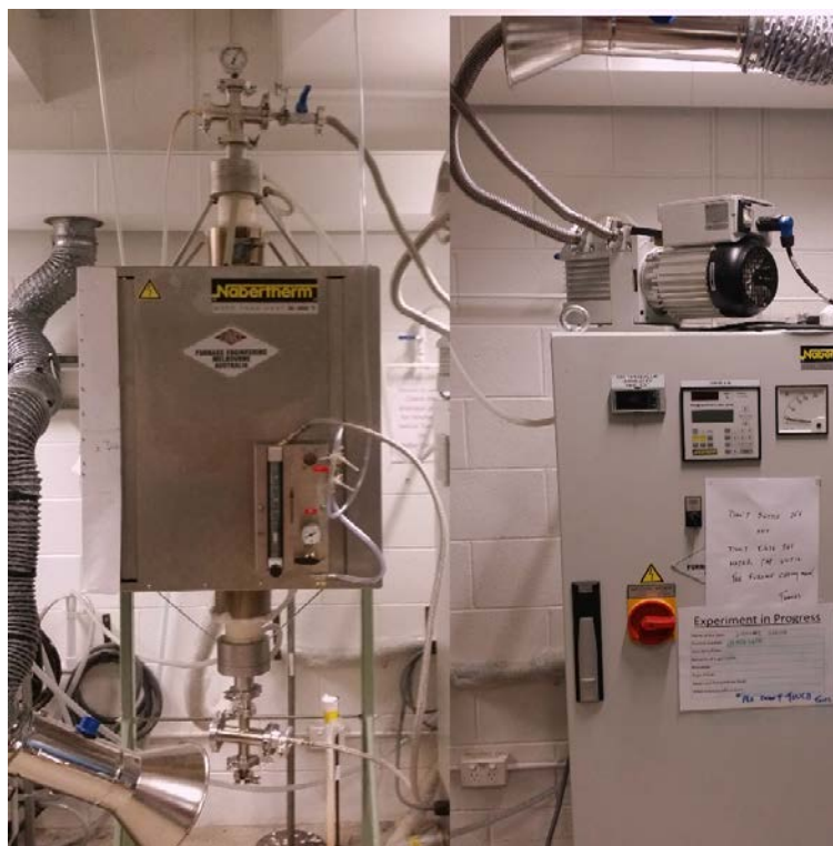
Figure A.3: Vertical tube furnace with controller temperature equipped with vacuum pump.
