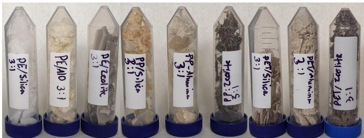
**Figure 6.3:** Colours of various metal oxide/waste plastic composites.
