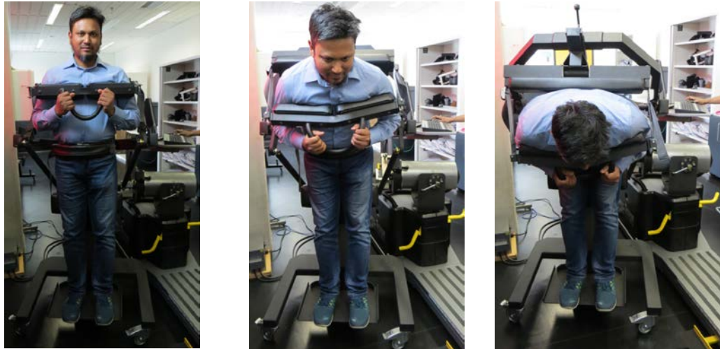
Figure 4.4 Trunk strength measurement in a laboratory settings
