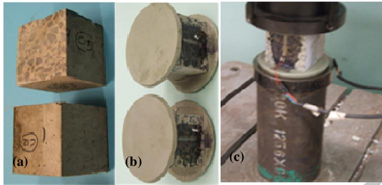
Fig.5: (a) concrete cubes, (b) prepared specimens for testing, (c) test set-up
