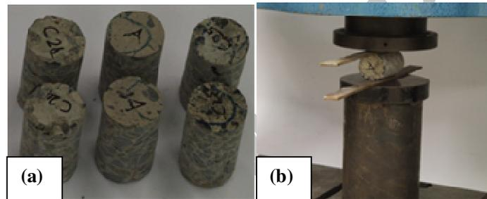
Fig.6: (a) Test samples, (b) Split-cylinder test set-up
