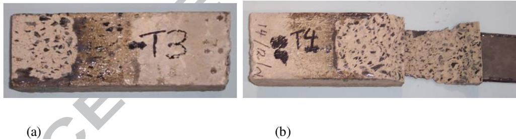
**Fig.2** Typical failure mode under ambient temperature; (a) bond length = 75 mm, (b) bond length  $\geq$  100 mm
