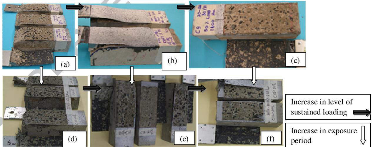
**Fig.9:** Failure mechanism,(a) 0% load, 1800 hrs, (b) 25%, 1800 hrs, (c) 50%, 1800 hrs,
