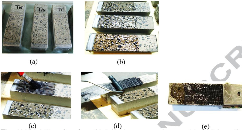
**Fig. 1**(a) Sand blasted surface (b) Primed concrete substrates (c) Applying adhesive on primed surface (d) Removing entrapped air bubbles and pressing (e) Prepared test specimens with gripping
