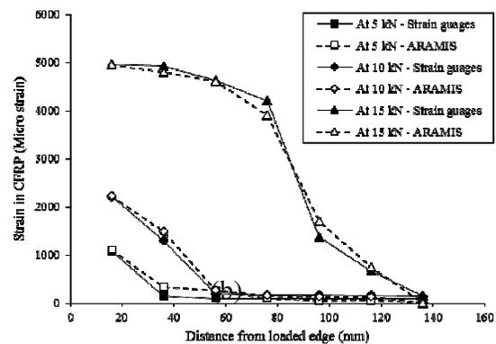
Fig. 7 (a) Failure pattern of control test specimens (b) Average strain distribution measured with strain gauges and ARAMIS photogrammetry technique
