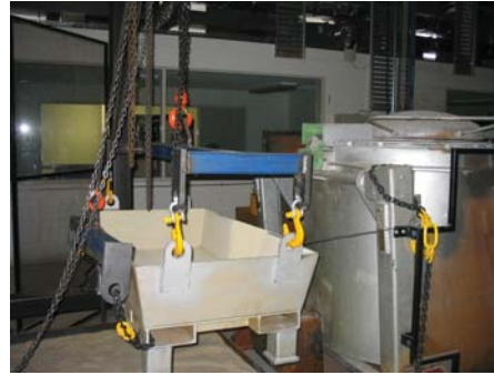
Fig. 2 500 kg tilting furnace and slung sow mould used for medium-scale pouring experiments.
