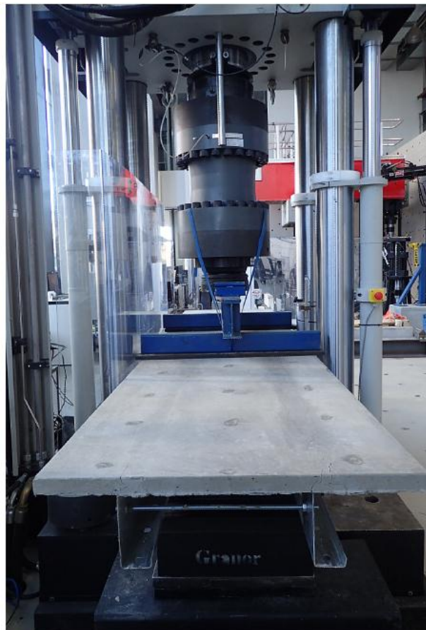
Figure 12-19: Different views of the four-point bending test setup
