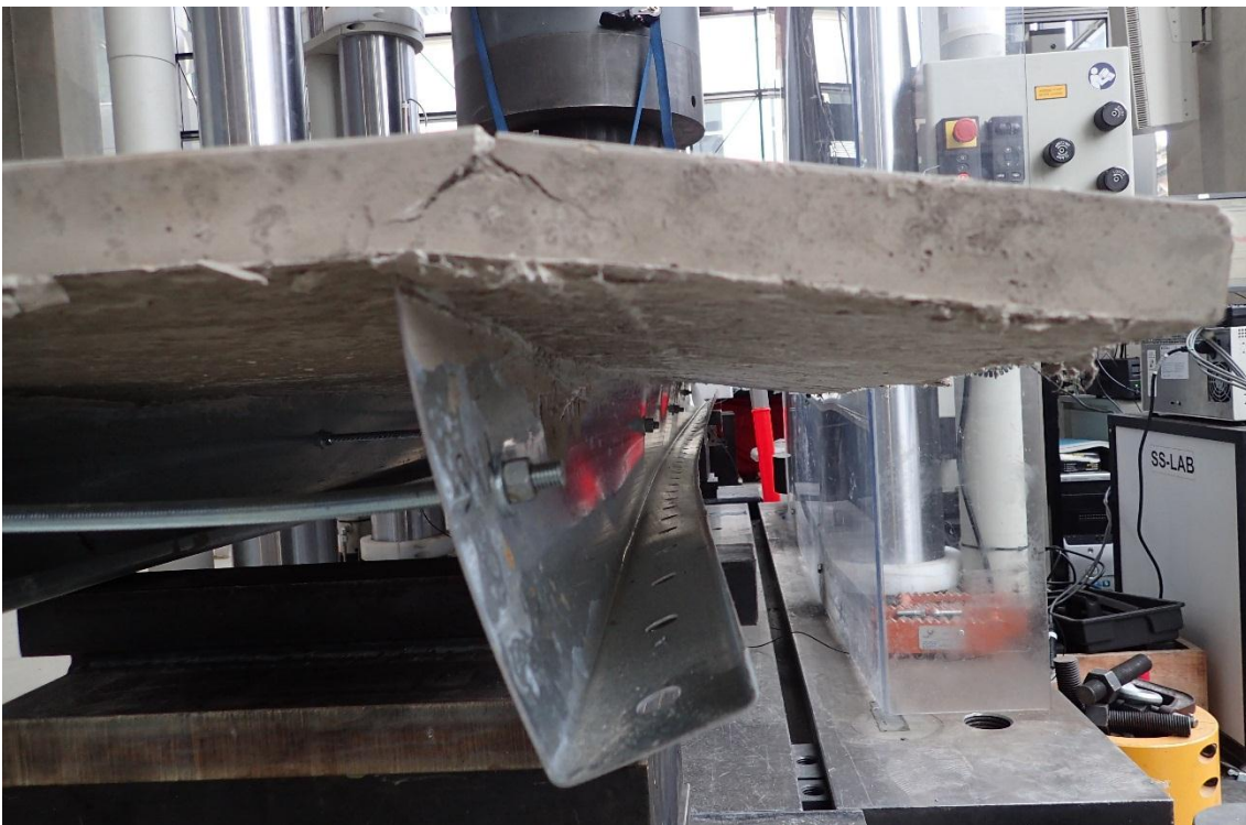
Figure 12-22: Elastic lateral torsional buckling of the C-sections
