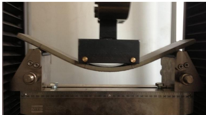
Figure 4-15: Very high ductile behavior of SHGC-Na-1 in bending
