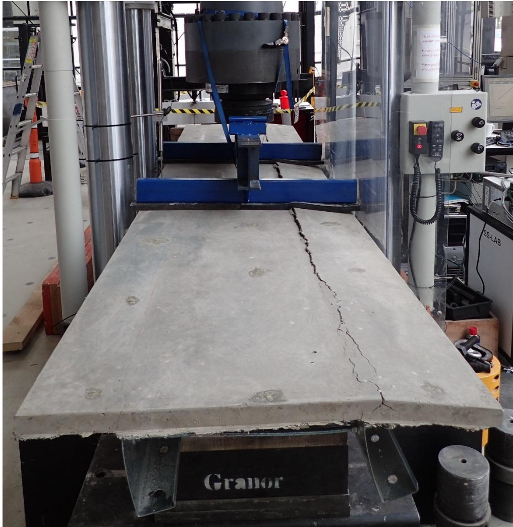
Figure 12-23: Development of long cracks on the top surface of the slab along the location of the top flange of one of the C-section
