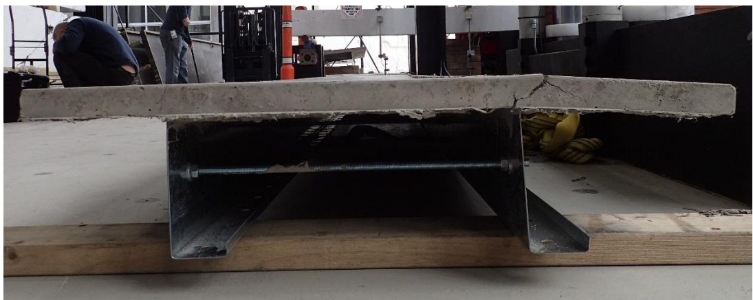
Figure 12-24: Return of C-sections to their original shape after unloading, indicating that all C-sections experienced “elastic” LTB
