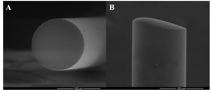
Figure 5. Examples of SEM images of SMF-28 fiber tip with 20° angle. The tip surface is clean and uniform (A), although a rounded upper edge was detected on the tip itself (B).
