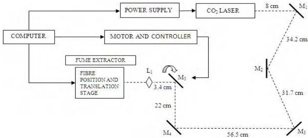
Figure 1. Laser cleaving system diagram.  $M_1$ ,  $M_2$ ,  $M_3$  and  $M_4$  are fixed mirrors while  $M_5$  is a rotating mirror;  $L_1$  is an aspherical lens. The dashed lines designate the beam path. The distances between the elements are expressed in cm.
