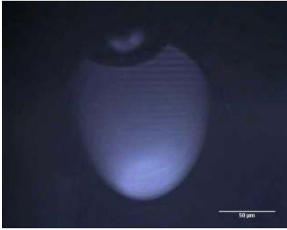
Figure 2. Example of the effects of uneven heating on the surface of a SMF-28 fiber. The cavity on the superior edge of the tip is caused by the fiber itself acting as a lens and focusing the laser beam to a small region. In this position, the deposited energy is higher than that on other parts of the tip surface.
