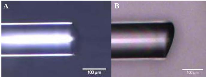
Figure 3. Example of SMF-28 fibers with 0° angle tip (A) and 20° angle tip (B). The round edge of the fiber is clearly visible in both samples. In particular in (A) it involves the entire tip surface, while in (B) it is confined to the superior edge of the tip.
