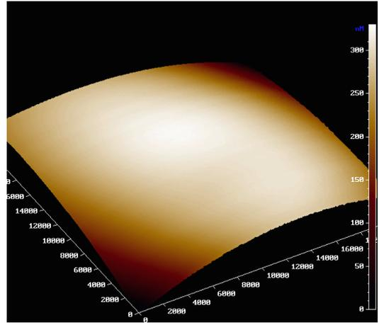
Figure 4. AFM image of an SMF-28 fiber tip cut with 0° angle. The curvature of the surface is clearly visible. The highest point of this curve is about 6 μm higher than the horizontal base plane of the surface.
