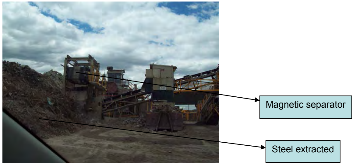
Figure 4.4: Steel extracted from RC
