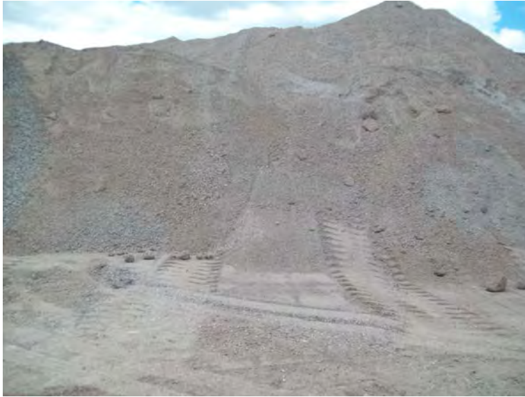
Figure 4.7: A dry crushed Concrete mix pile
