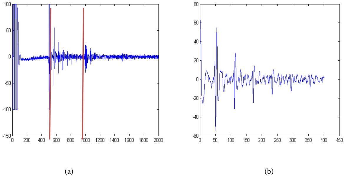
123 **Fig.1.** (a) An example of a ultrasonic signal gated on the captured A-scan signal. (b) A signal singled out.
