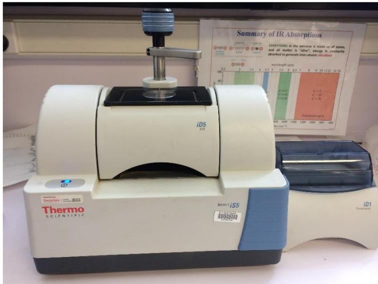
Fig. 4-2. Nicolet™ iS5 Spectrometer for FT-IR test
