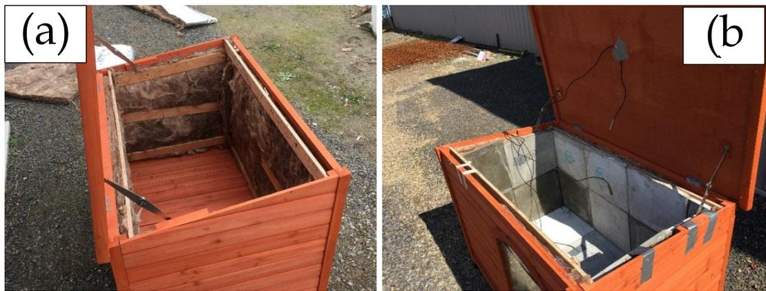
Fig. 7-3. Test hut set up (a) installation of insulation to the interior walls (b) PCMCB installed to the interior surfaces
