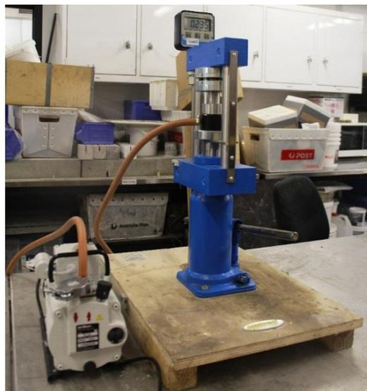
Fig. 6-2. Pelletizing of PCM composite discs containing carbon additives
