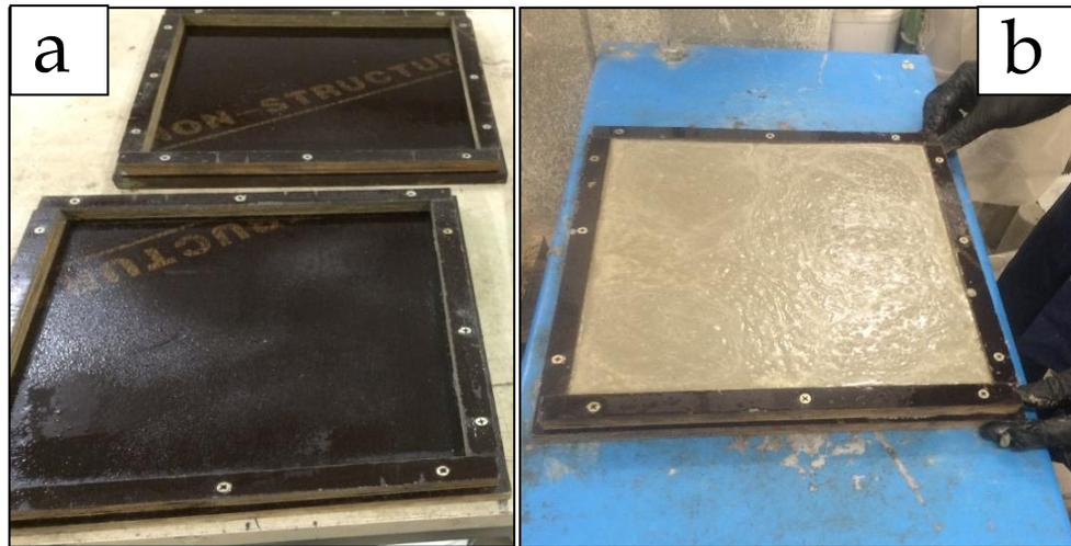
Fig. 4-1. TESC panels for thermal performance test (a) timber molds (b) compaction of TESC using mechanical vibration
