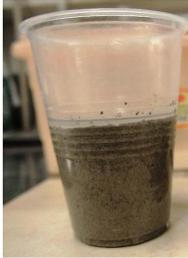
Fig. 3-5. Cementitious composite mixture poured in transparent cylindrical cup
