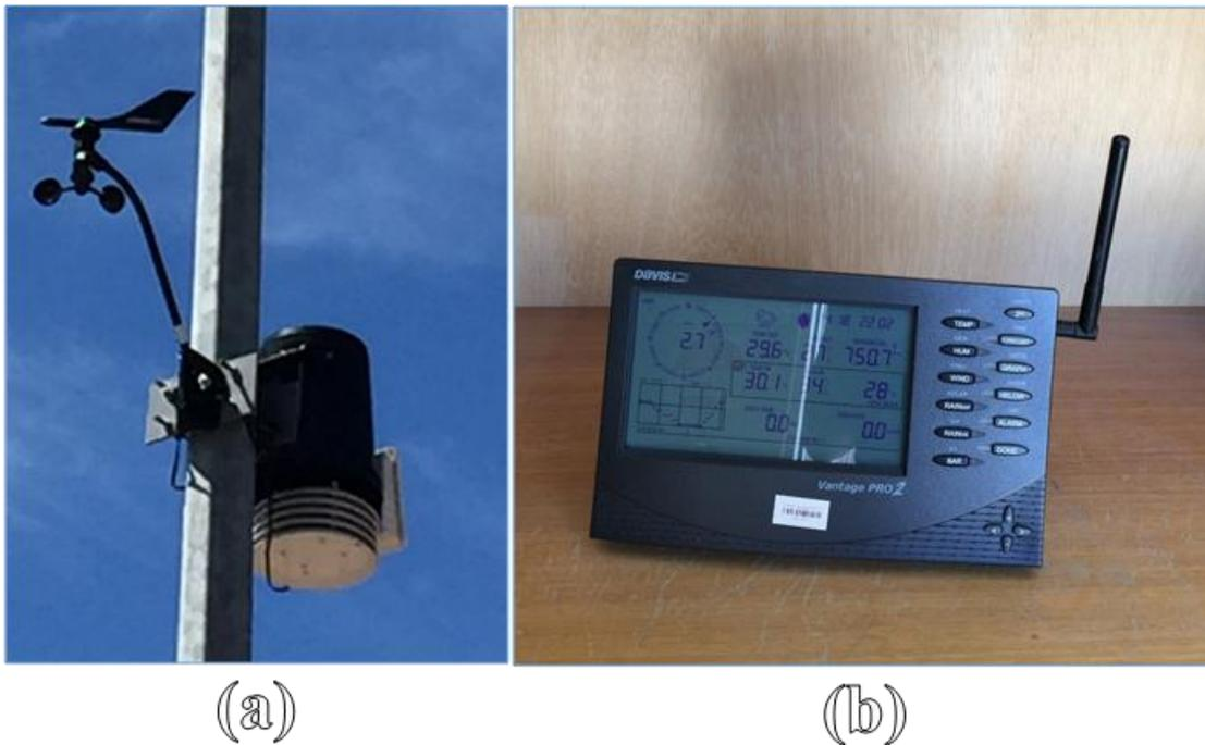
Fig. 7-5. Meteorological station at the test site (a) weather station (b) console unit
