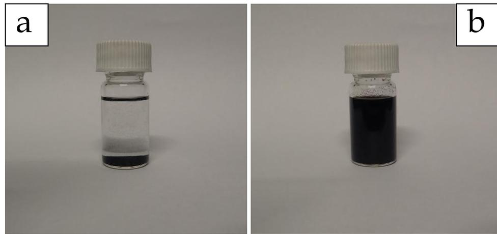
Fig. 6-1. Dispersion of CNT in acetone using ultrasonic bath (a) before dispersion (b) after dispersion
