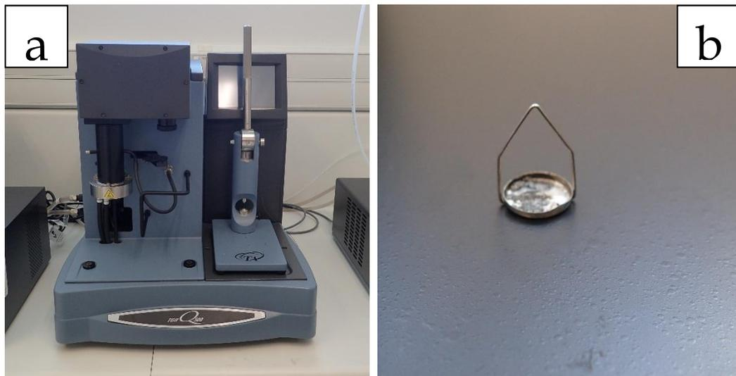
Fig. 4-3. Thermo-gravimetric analysis (a) TGA apparatus (b) ceramic pan
