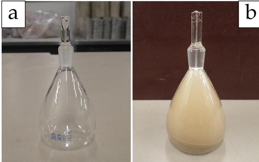
Fig. 4-4. Density bottle test (a) water pycnometer (b) sand slurry filled with water
