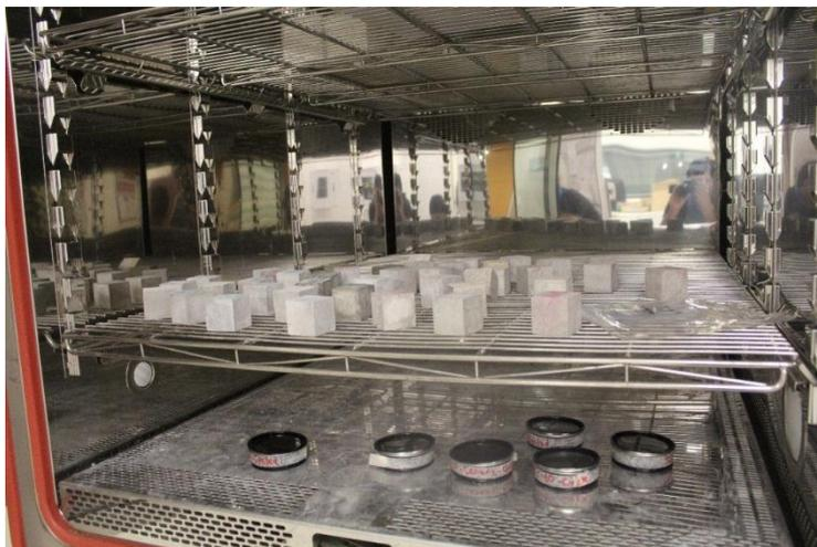
Fig. 5-6. Specimens subjected to accelerated thermal cycles test
