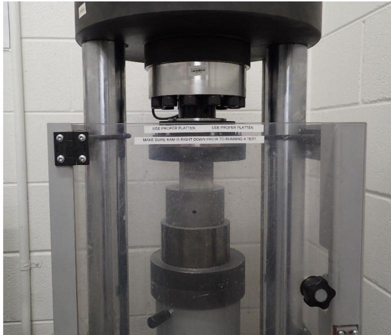
Fig. 4-5. Technotest C030/2T compressive strength testing machine
