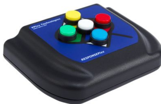
Figure 5.2. RESPONSEixx button box. Pressing the green button indicated numerosity estimation judgements of 'more dots', and pressing the red button indicated numerosity estimation judgements of 'fewer dots'. The button responses and response times per trial were recorded onto an excel spreadsheet.
