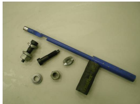
Figure 2 Original Ajax blind bolts and tool
