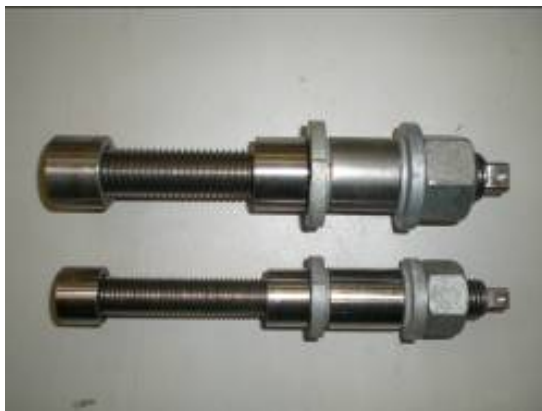
Figure 1 Modified blind bolts with extensions
