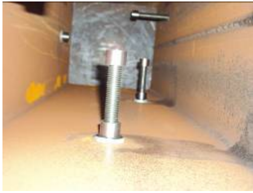
Figure 5 Blind bolts in the square hollow section Figure 6 Test setup on SHS column
