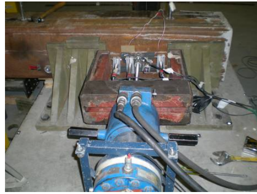
Figure 5 Blind bolts in the square hollow section Figure 6 Test setup on SHS column
