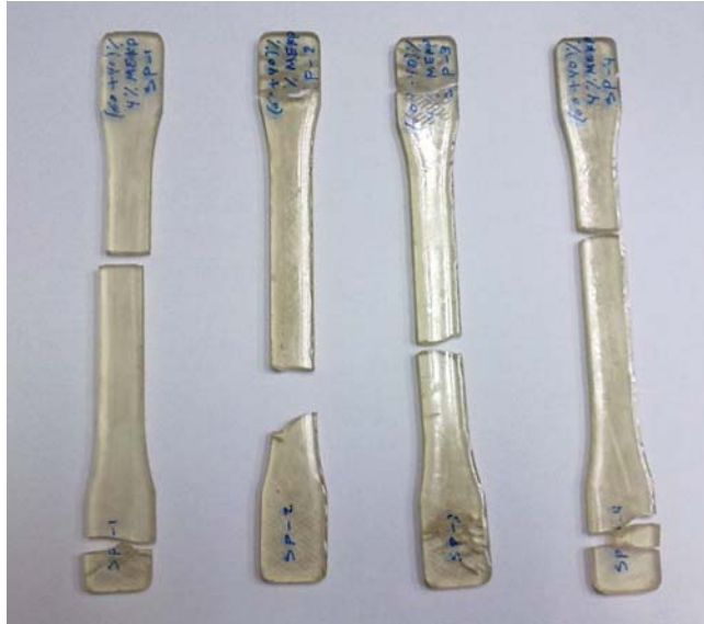
Figure 4.13 Photograph of the failed tensile test specimens for unsaturated polyester
