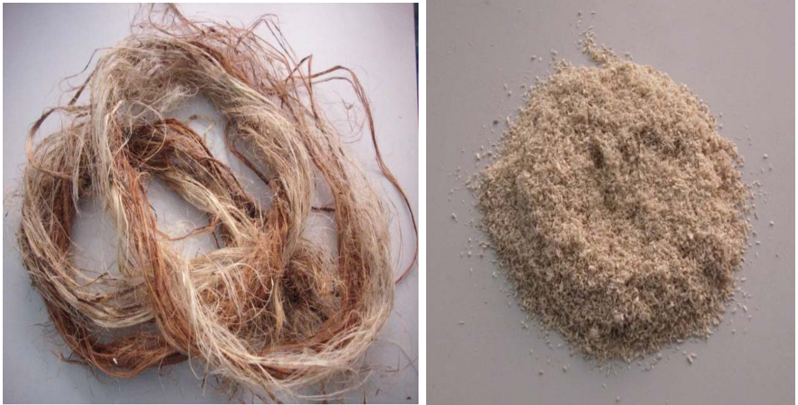
Figure 2.3 The long and short fibers, Kenaf Natural Fiber Industries Sdn. Bhd. http://www.kenaffiber.com
