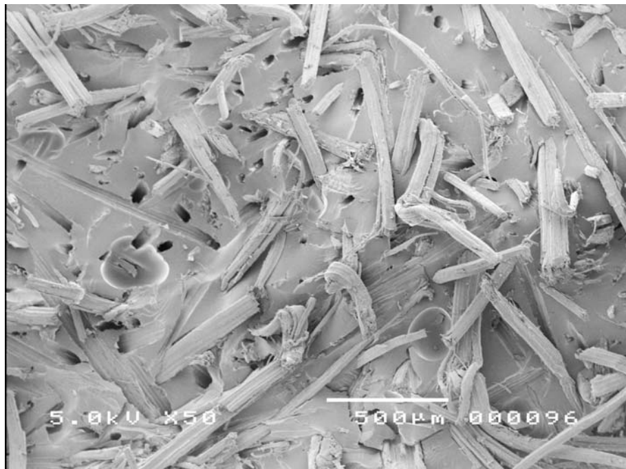
Figure 6.35 The SEM micrograph of bending fractured surface of the composites: a) 25°C at 37 days, b) 50°C at 37 days
